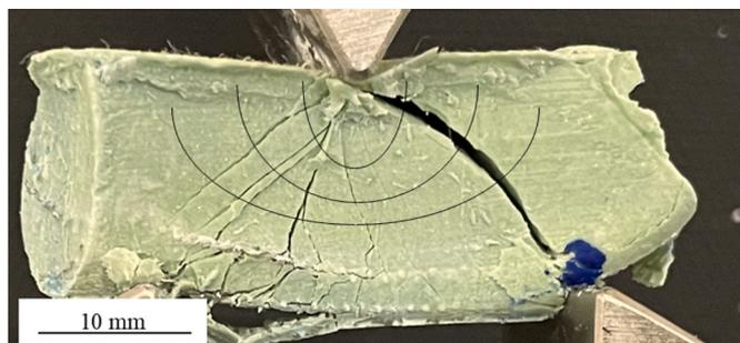
Fig. 7. Snapshot of S2 sample loading in three-point bending showing the crack pattern, overlaid with the trajectories of principal tensile stresses.
