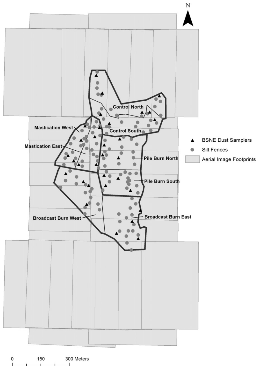
Figure 2. Forty overlapping aerial photographs were acquired for the study area in June 2009 and 2010. Field measurements of sediment flux were made using Big Spring Number Eight wind-aspirated dust samplers ( n = 32 ) and small silt fences ( n = 120 ) within the three treatment areas and control area. The map also shows treatment and control areas divided into sub-treatments, which were used to estimate average bulk density and local precision error thresholds.
