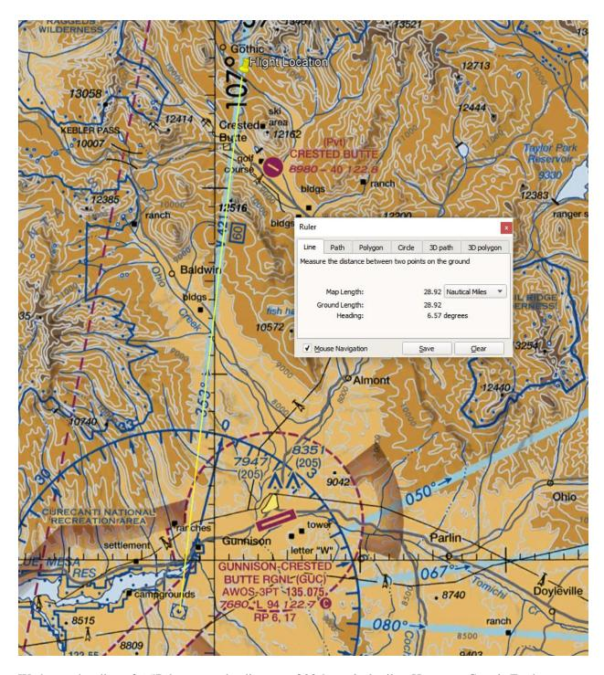
We have a heading of 6.57 degrees and a distance of 28.9 nautical miles. However, Google Earth measures headings relative to true north, and VORs are oriented relative to magnetic north. To make this conversion, we look for the nearest line of constant magnetic variation (again reference the airspace guide for more information). We find that the variation is about 8.5 degrees east. Easterly variation is subtracted, so we end up with a heading of about 358 degrees.
