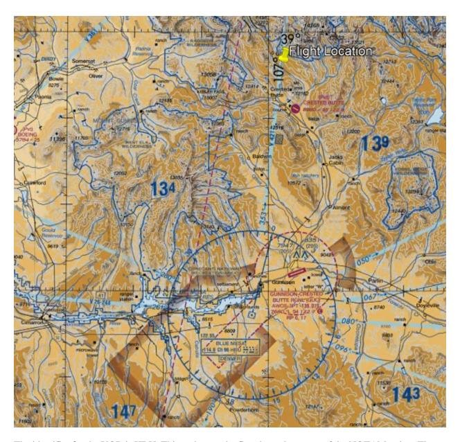
The identifier for the VOR is HBU. This makes up the first three characters of the NOTAM string. The next information that is needed is the radial and distance. Find this by using the ruler tool and measuring *from* the VOR *to* the flight location. This is what Google Earth returns:
