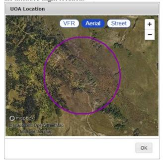
It is important to not make the radius larger than is needed. Increasing the radius to account for limited precision in defining the center point is acceptable, but in general, keep the radius to the minimum required value. An example of an unacceptable radius would be using something like 1nm for flying a small multirotor – VLOS will run out well before 1nm, and this NOTAM would overstate the impact of our operations on the NAS.
