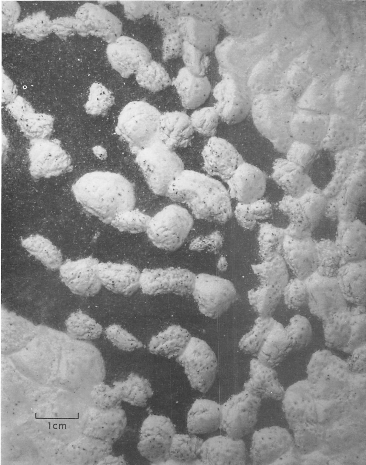
Figure 11. Miniature sorted nets produced by jarring a container of clay, settled from an aqueous suspension, and covered with a thin surface layer of sand.
