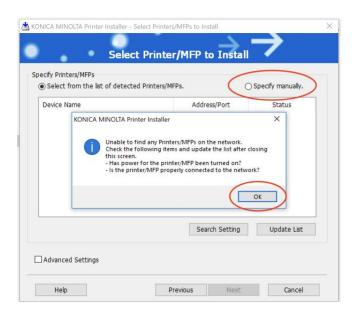
Step 4B: If you need to add it manually, after clicking on "Specify Manually", you will click on middle radio button under the "Network" options that says "IPv4, IPv6 address/Local Host Name", then enter the IP for the system you want to install, see IPs in Step 4A above:
