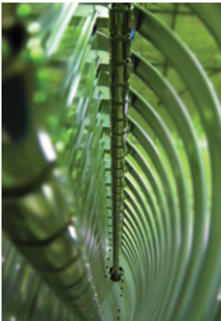
The 3 MV Electrostatic Accelerator (above) is the largest dust accelerator in the world and is available for use by the lunar, space and plasma physics communities. Photo © Keith Drake.
