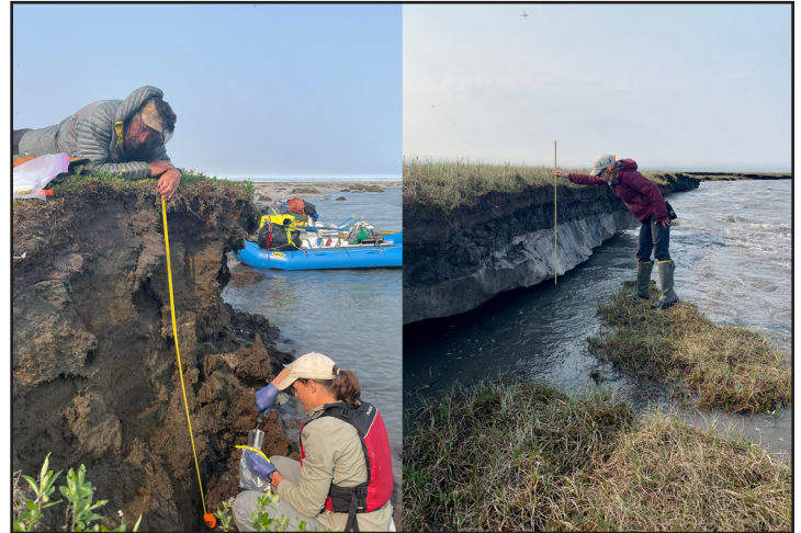
Taking measurements of peaty and icy riverbanks being thermally eroded in the Canning delta (photos Overeem and Repasch).
