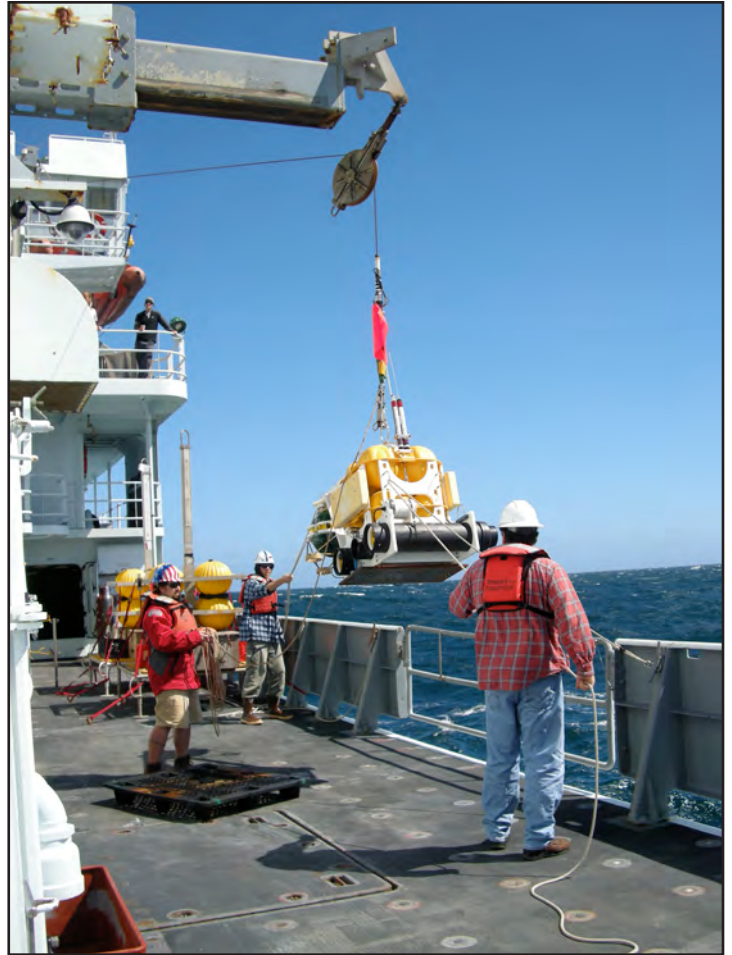
Ocean Bottom Seismometer package being deployed offshore New Zealand, February 2009. Geological Sciences graduate student David Culp and professors Peter Molnar and Anne Sheehan and participated in the month long research cruise and deployment.
