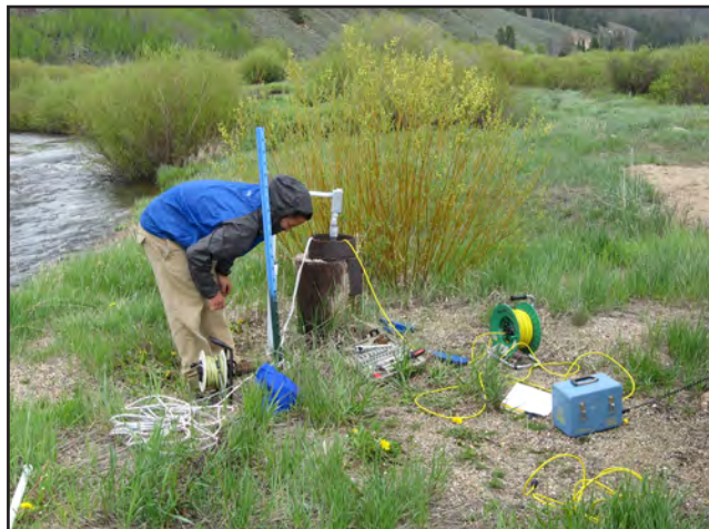
Graduate Student Alex McCaffree is monitoring groundwater level recovering readings during an aquifer permeability
