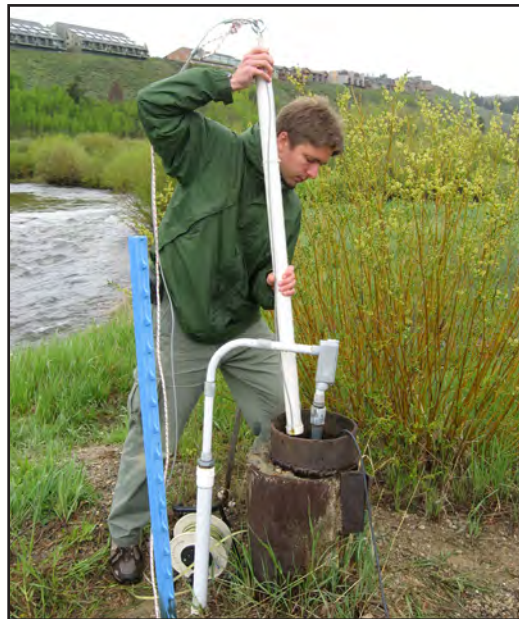
Graduate Student Brent Aigler lowering a slug into the well to start an aquifer permeability test in Fraser CO
