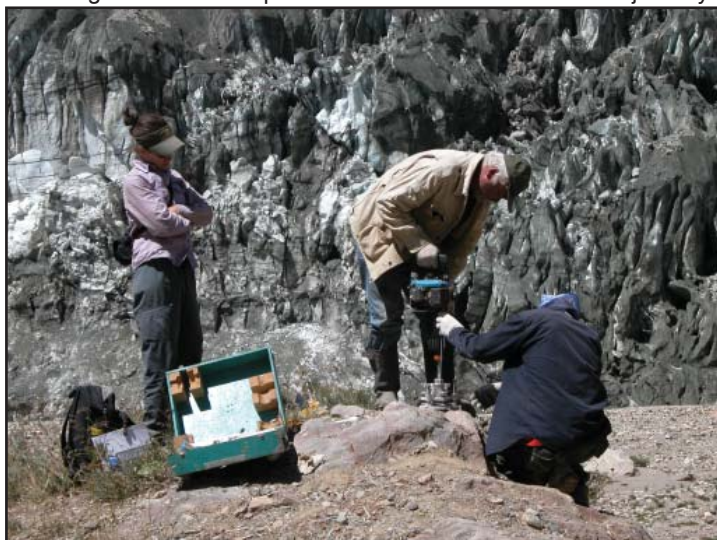
Installing a GPS control point at the eastern end of the Vanj Valley
