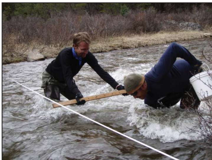
Greg Tucker and Nate Bradley planting radio-tagged tracer stones in the bed of Halfmoon Creek, near Leadville, May 2007. Tracking the motion of these clasts over time will reveal the pattern of dispersion and provide a test of mathematical models. The project is supported by an Innovative Research Grant from CIRES.
