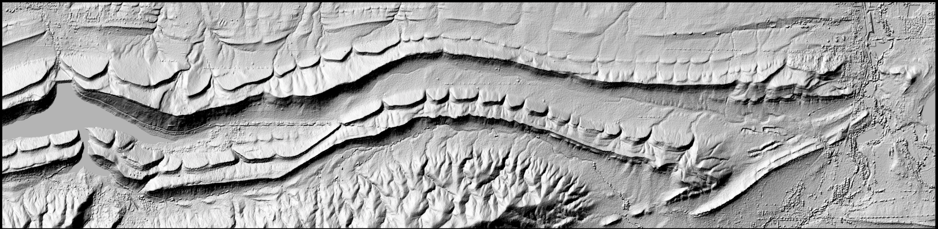
Shaded relief map derived from interferometric side aperture radar between Ft. Collins and Loveland. The image is based on a 5 meter digital elevation model of the Front Range donated to the Geology department by Intrasearch Corporation of Denver. The images resolve individual houses and large trees, allowing field students to visualize geologic structures and topography at very fine scales. Additional images from Ft Collins to Castle Rock are archived in the Jerry Crail Johnson map library. Images created by Sean Sundermann, Alex Tate and Ryan Tolene.
