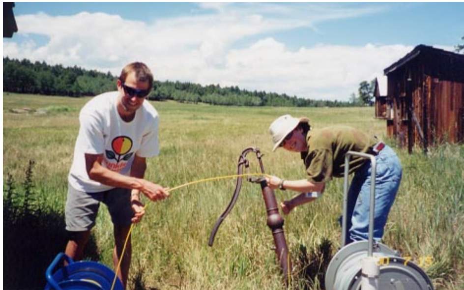
Steve Shultz and Stephanie Tomusiak are conducting aquifer tests in Turkey Creek, CO
