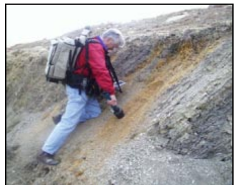
Alex Goetz making a field spectral reflectance measurement on an outcrop of the near-vertically-dipping Pierre Shale near Morrison, CO.
