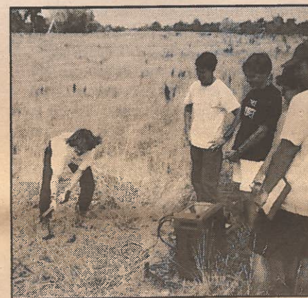
Seismic refraction experiment near Boulder Creek. Prof. Anne Sheehan hits the ground with a sledgehammer in order to generate seismic waves which are reflected and refracted off various subsurface rock layers. The goal of this experiment was to determine depth to the water table and bedrock.
