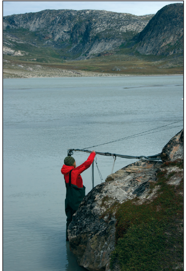
Associate Professor Irina Overeem installing turbidity and stage measurement station in Greenland Delta.
