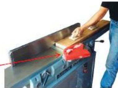
Self-adjusting blade guard
