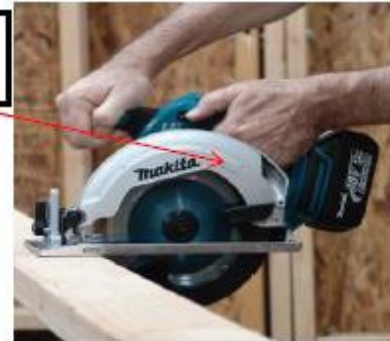
Self-adjusting blade guard
