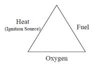
For ignition to occur a fire needs three things: heat, fuel and oxygen. A properly used extinguisher will smother the burning surface, lower the temperature and/or remove the oxygen, thus extinguishing the fire.
