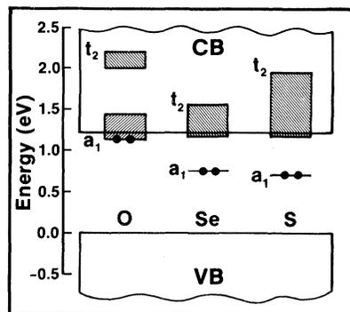
FIG. 3. Energies of the  $a_1$  and  $t_2$  gap levels and resonances (shaded) for substitutional chalcogen impurities in silicon.
