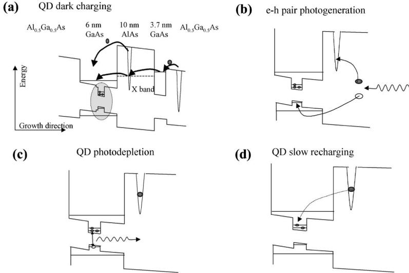
FIG. 1. Schematic description of the mixed type SAQD sample. (a) Initial charging of the QD with electrons from ionized donors, (b)  $e$ - $h$  pair photogeneration, (c) QD photodepletion, and (d) QD slow recharging by the captured electron from the ionized donor.
