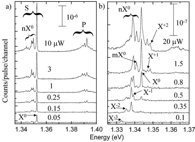
FIG. 2. Picosecond pulse excited photoluminescence spectra of single QD's for increasing excitation intensities. (a) From a charge-neutral QD (the control sample A) and (b) from a charged QD (mixed type sample B). The discrete PL lines due to the recombination of neutral excitons ( $X^0$ ,  $nX^0$ ), negatively charged ( $X^{-i}$ ) and positively charged ( $X^{+i}$ ) excitons are marked in the figures.
