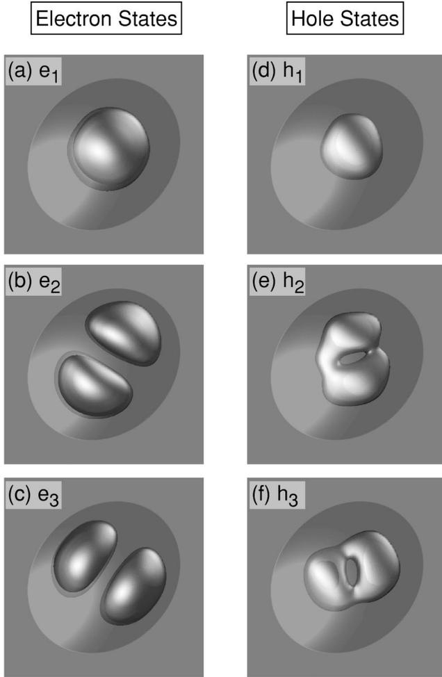
FIG. 4. Top view of the calculated single electron and hole wave functions squared for the SAQD under study. The isosurfaces contain 75% of the total charge. The pseudopotential calculations use the linear combination of bulk bands method (Ref. 29). Note that the spatial extent of the electron wave function is larger than that of the hole.
