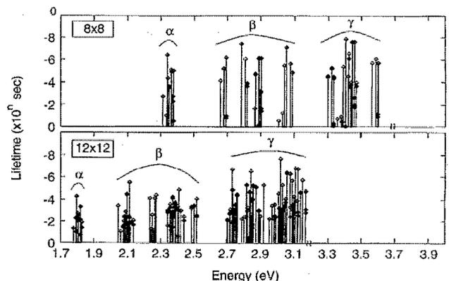
FIG. 3. Calculated radiative transition lifetime from the four highest VB states as functions of the transition energy.
