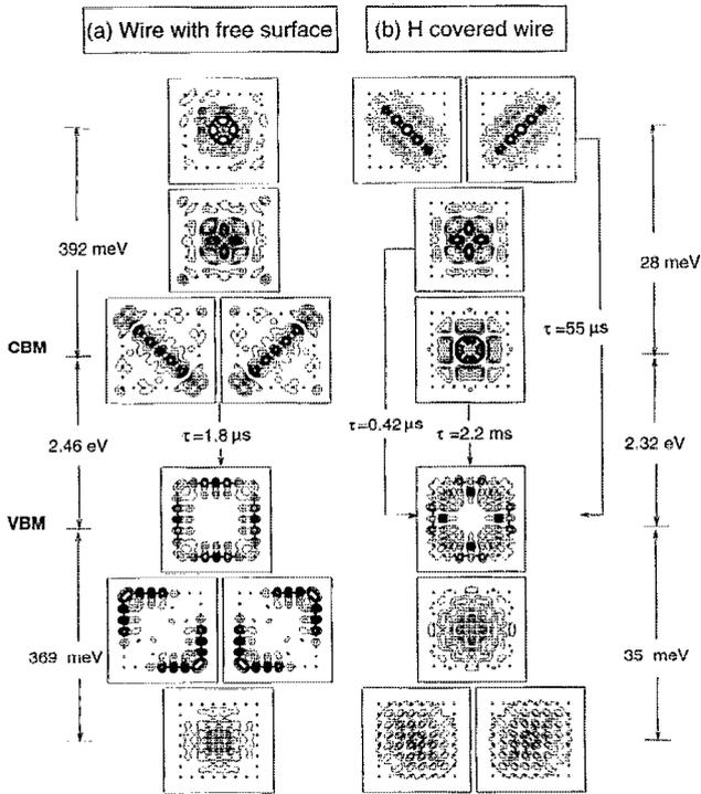
FIG. 1. z-direction averaged wave-function squares, energy separations, and lifetimes for the near band-gap states. The dots denote positions of outer Si atoms.
