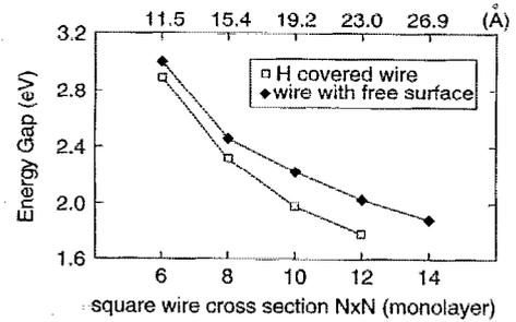
FIG. 2. Dependence of the band gap on the wire size. For the wire with free surfaces we consider only intrinsic states.
