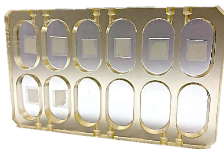
Figure 6. 12-Well BioCell – BioServe’s 12-Well BioCell loaded with 8 1x1x.1cm silicone coupons.
