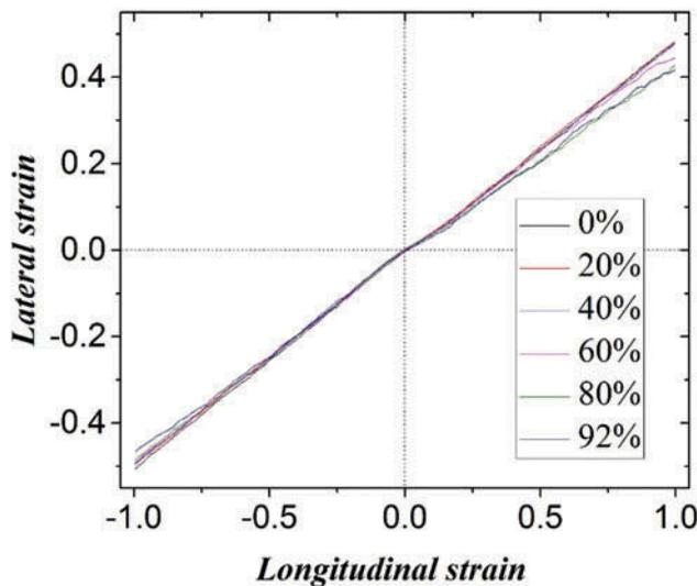
**Figure 11.** Lateral versus longitudinal strain curves of the differently cross-linked systems at 300 K.
