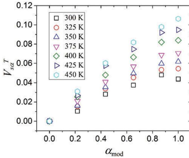
Figure 7. Volume shrinkage  $V_{sa}^T$  versus  $\alpha_{mod}$  at various temperatures.
