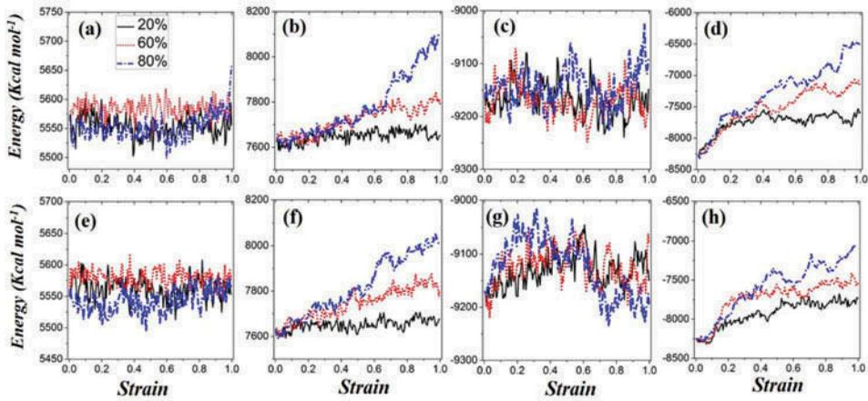
**Figure 10.** Evolution of different energy contributions including bond stretching, bending, torsional, and pairwise (LJ + coulombic) interaction (a)–(d) under tension and (e)–(h) under compression.
