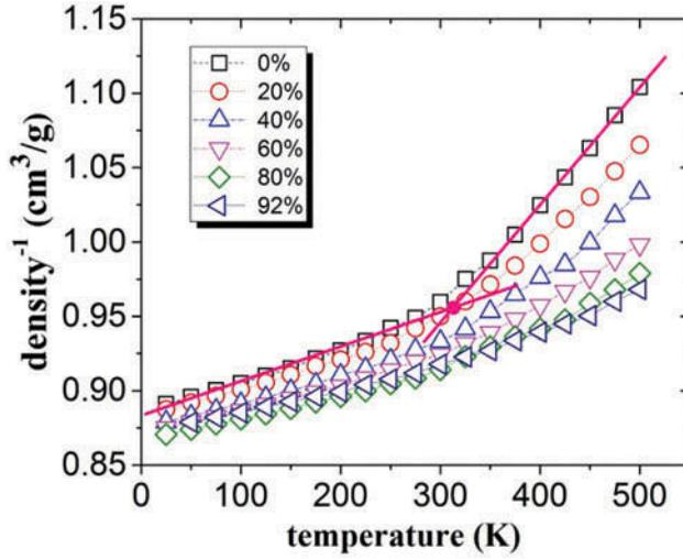
**Figure 6.** Variation in specific volume at various temperatures of differently cross-linked resin systems.
