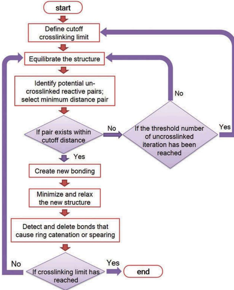
Figure 3. Flowchart that demonstrates the cross-linking algorithm.
