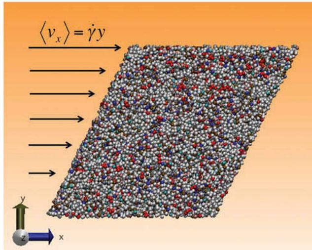
**Figure 5.** Schematic of the Couette flow model of the epoxy resin system.
