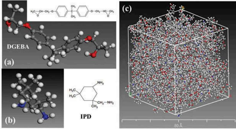
**Figure 1.** Structure of (a) resin, (b) cross-linker molecules, and (c) and resin system built in the Materials Studio package.
