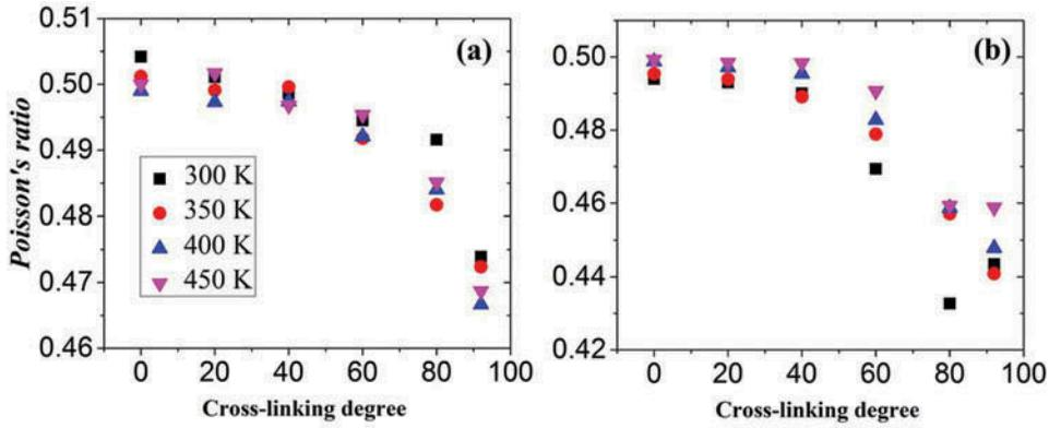
Figure 12. Poisson's ratio under compression (a) and tension (b) for the differently cross-linked systems at various temperatures.
