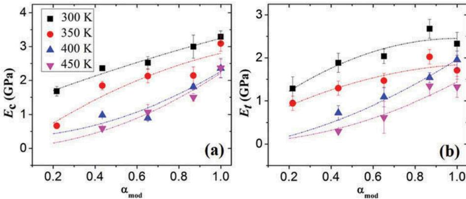
**Figure 14.** Elastic modulus  $E$  versus  $\alpha_{\text{mod}}$  under (a) compression and (b) tension at various temperatures.
