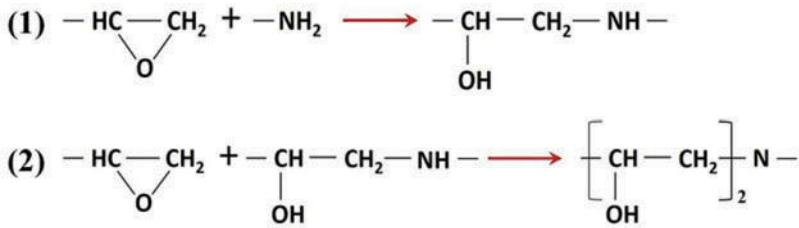
Figure 2. Two principal reactions involved in the curing of a diamine with a diepoxide.
