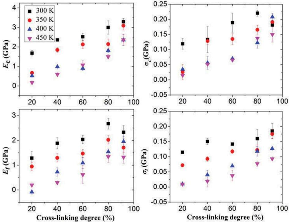
Figure 13. Extracted Young's modulus ( $E$ ) and yield stress ( $\sigma$ ) under compression and tension for the differently cross-linked systems at various temperatures.
