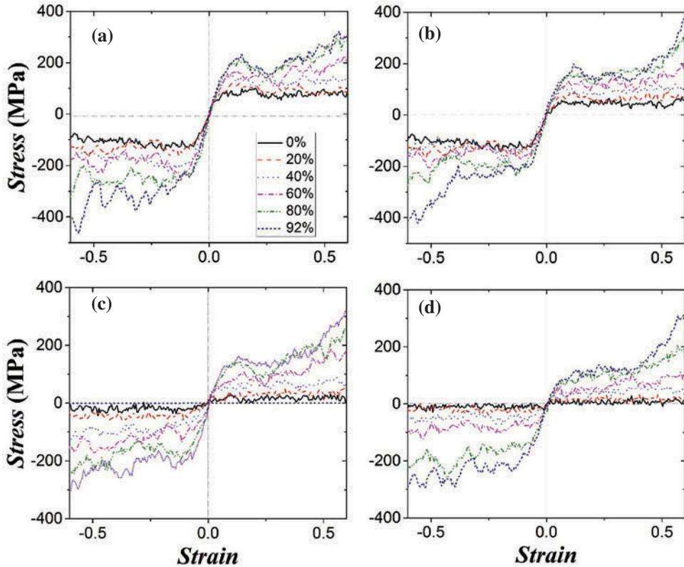
**Figure 9.** True stress–strain curves of the differently cross-linked systems at (a) 300 K, (b) 350 K, (c) 400 K, and (d) 450 K.
