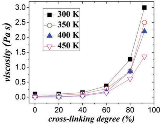
**Figure 15.** Variation in viscosity with cross-linking degree at different temperatures.
