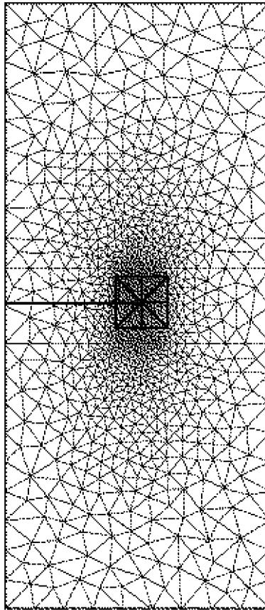
Figure 10. Basic and overlaid meshes for edge-cracked specimen under uniform tension and shear.
