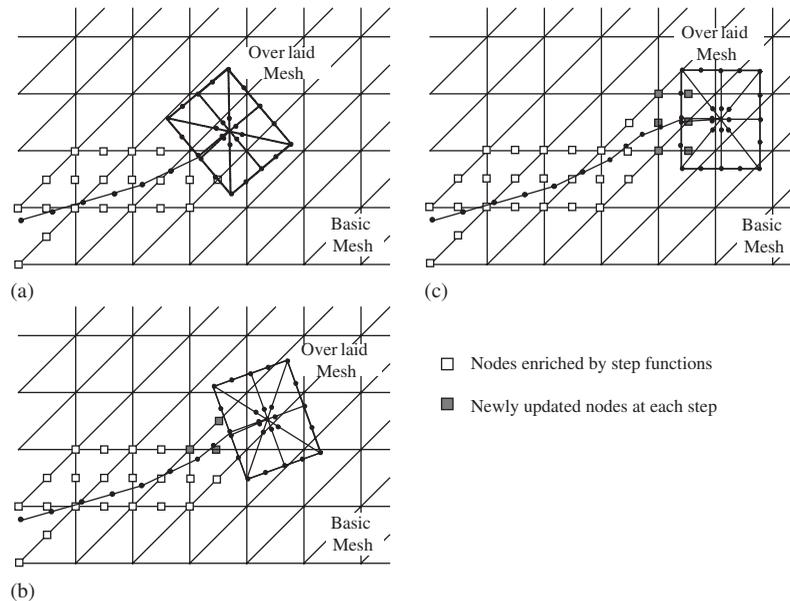
Figure 5. Modelling of crack propagation in the XS-FEM; an overlaid mesh is translated or rotated and enriched nodes are updated in a basic mesh at steps (a)–(c).
