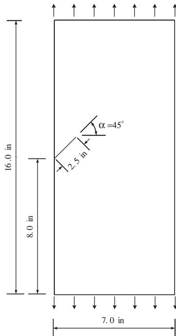
Figure 12. Problem description for modelling growth of slanted edge crack in a plate under tension.
