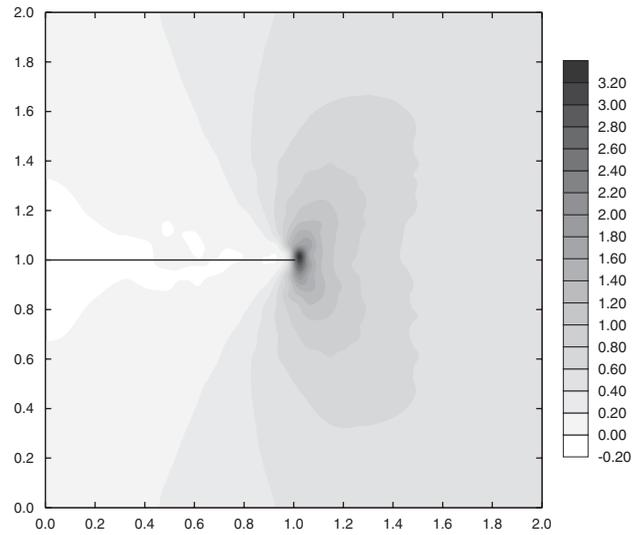
Figure 8. Stress ( $\sigma_y$ ) contour plot of square patch with near-tip fields (unit: psi).
