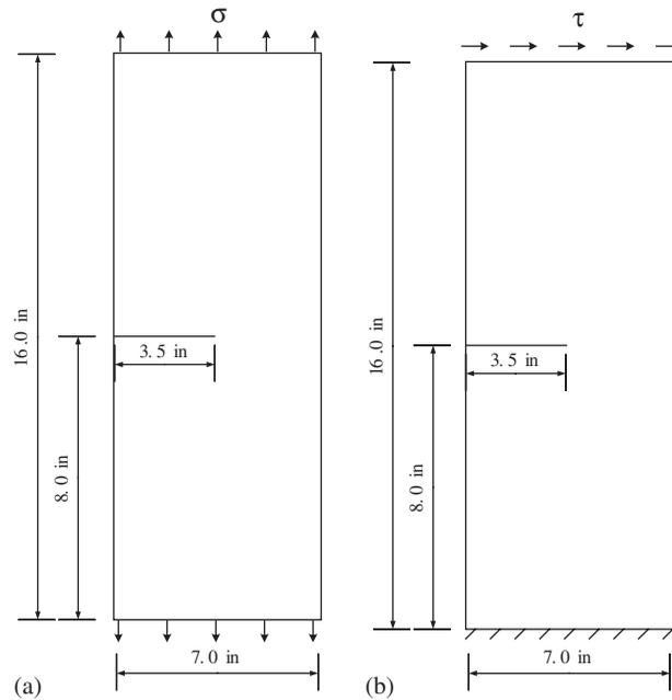
Figure 9. Problem illustrations: (a) edge-cracked specimen under tension; and (b) edge-cracked specimen under shear.
