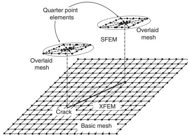
Figure 2. Mesh discretization of the basic and overlaid domains in the XS-FEM; the near-tip field of the overlaid domain is modelled by quarter point elements and the rest of the crack is treated by the XFEM on the basic mesh.
