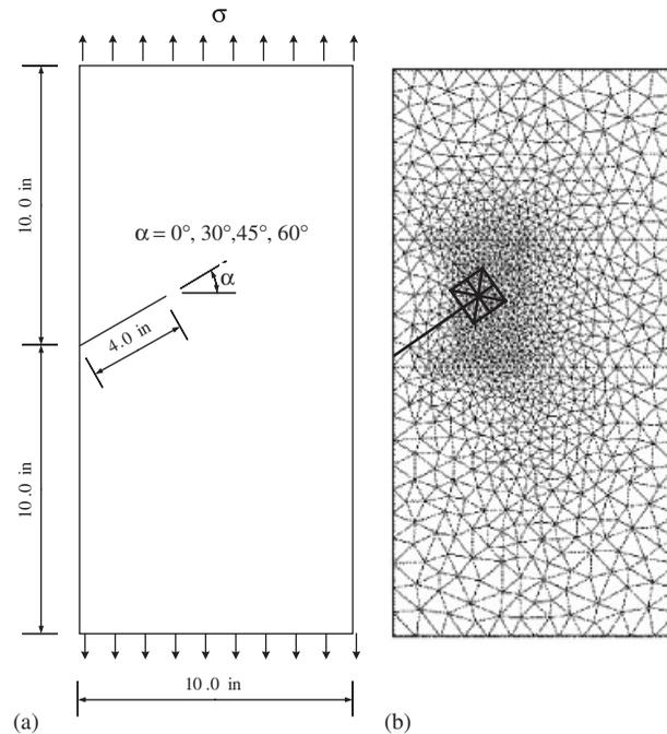
Figure 11. Edge crack with variation of slant angles under tension: (a) problem description; and (b) basic and overlaid meshes.
