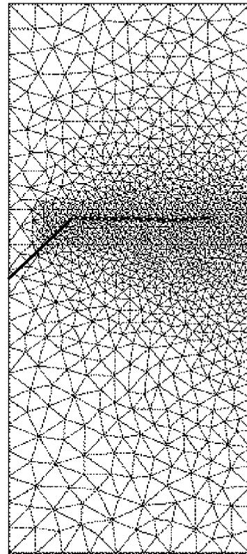
Figure 13. Final configuration of slanted edge crack after growing under tension.
