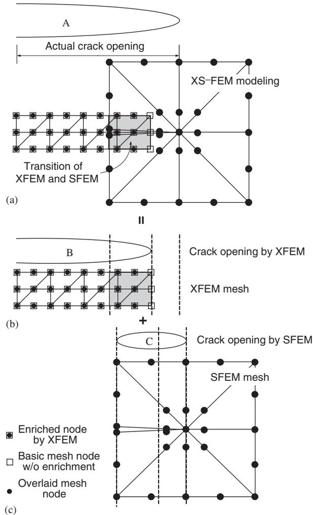
Figure 4. Modelling of a crack opening displacement ( $A = B + C$ ): (a) actual crack opening and its modelling by XS-FEM; (b) crack opening by discontinuous enrichment of the XFEM on the basic mesh; and (c) crack opening by the SFEM on the overlaid mesh.
