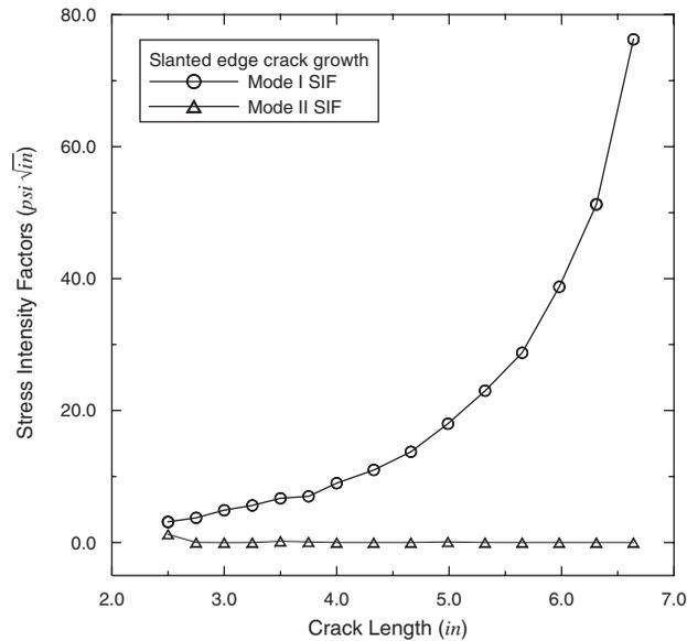
Figure 14. Modes I and II stress intensity factors as a function of the length of the crack.
