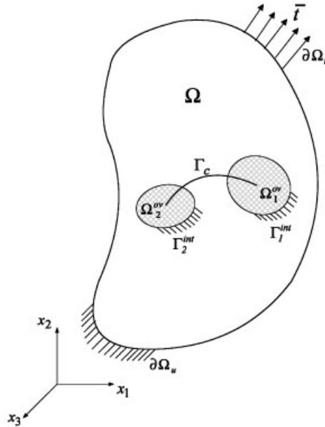
Figure 1. Basic domain ( $\Omega$ ) and overlaid domains ( $\Omega_i^{ov}$ ,  $i = 1, 2$ ) in the XS-FEM.
