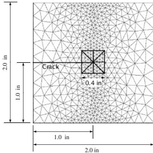
Figure 6. A square patch with near-tip field and the mesh structure.
