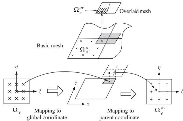
Figure 3. Mapping procedure from the parent co-ordinate  $(\zeta, \eta)$  of basic mesh to the other parent co-ordinate  $(\zeta', \eta')$  of overlaid mesh for the quadrature of weak form and the measurement of displacement and stress fields.
