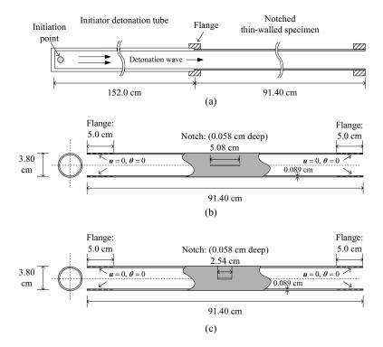
Fig. 8 Setup for the notched cylinder fracture under internal detonation pressure [16]: (a) total experiment assembly, (b) notched thin-walled specimen for shot 7, and (c) notched thin-walled specimen for shot 4
