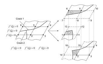
Fig. 5 The decomposition of an element into three elements  $e_1$ ,  $e_2$ , and  $e_3$  to model crack branching; solid and hollow circles denote the original nodes and the added phantom nodes, respectively
