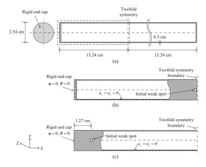
Fig. 17 Setup for cylinder fracture with an initial weak spot: (*a*) only half of the cylinder is modeled due to the twofold symmetry, (*b*) cylinder with an initial weak spot at the center of the cylinder, and (*c*) cylinder with an initial weak spot close to the end cap
