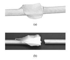
Fig. 11 Comparison of the final deformed shape between (*a*) the simulation result and (*b*) the experimental result (shot 7) [16,25]
