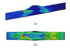
Fig. 10 Evolution of crack opening at time  $t=256.86 \ \mu s$  along with distribution of effective plastic stress: (*a*) side view and (*b*) top view
