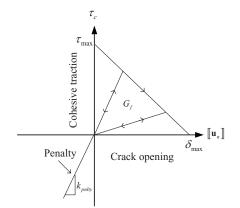
Fig. 7 Schematic showing of a linear cohesive law: the area under curve is the fracture energy,  $G_f$
