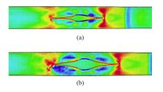
Fig. 13 Evolution of crack and distributions of effective plastic stress at time times (*a*)  $t=231.41 \ \mu$ s and (*b*)  $t=239.05 \ \mu$ s. Note that finite element nodes are plotted and crack paths are explicitly marked.
