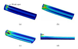
Fig. 18 The computed final deformed shape along with marked opened crack surfaces: (a) perspective view and (b) axial view
