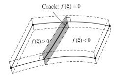
Fig. 2 Representation of discontinuity in the reference configuration by a level set implicit function  $f(\xi)$  in the shell midsurface
