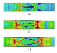
Fig. 9 Evolution of crack paths and distributions of effective plastic stress at different time steps: (a)  $t=213.55 \ \mu$ s, (b)  $t=228.61 \ \mu$ s, and (c)  $t=238.01 \ \mu$ s. Note that finite element nodes are plotted and crack paths are explicitly marked.
