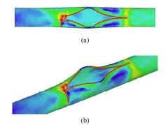
Fig. 15 Evolution of crack and distributions of effective plastic stress at time  $t=261.98 \ \mu$ s: (a) top view and (b) side view
