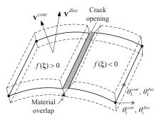
Fig. 3 Nomenclature of a fractured shell descriptions: incompatible material overlaps occurred at the bottom surface due to crack opening
