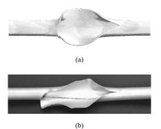
Fig. 16 Comparison of the final deformed shape between (*a*) the simulation result and (*b*) the experimental result (shot 4) [16,25]
