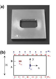
Fig. 1. The novel experimental set-up: (a) optical photograph of the frame and a glass specimen, and (b) schematic presentation of the specimen, boundary conditions, dimensions, and the location of the two typical precracks. The two strain gauges for the calibration procedure are also shown.
