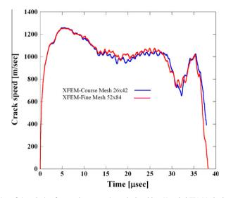
Fig. 9. Crack velocity as a function of time during fast crack propagation calculated by eXtended FEA Method using the coarse and fine meshes.
