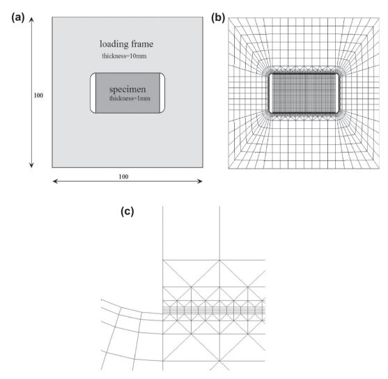
**Fig. 2.** The loading system as a 2D problem: (a) the equivalent 2D geometry substituting the 3D assembly, (b) the finite element mesh used by Franc2D code, and (c) details of the zone containing the frame, the specimen and the epoxy.
