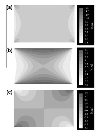
**Fig. 4.** The calculated contour levels of stress fields: (a)  $\sigma_{yy}$ , (b)  $\sigma_{xx}$ , and (c)  $\sigma_{xy}$  in an unnotched specimen. Note the even distribution and the dominance of  $\sigma_{yy}$  over  $\sigma_{xx}$  and  $\sigma_{xy}$ .
