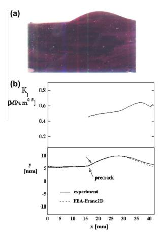
Fig. 6. The experimental and numerical crack path of a slow crack: (a) optical photograph of the fractured soda lime glass specimen, and (b) the experimental and numerical path (Franc2D) selected by a slow crack.
