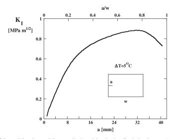
**Fig. 5.** The SIF  $K_l$  as a function of the crack length, a, and the normalized crack length, a/w, of a single edge, type A crack (see Fig. 1c) for the assembly materials described in Table 1.
