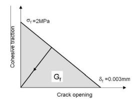
**Fig. 7.** Linear cohesive law; the area under the cohesive law curve is the same as the fracture energy  $G_{fr}$
