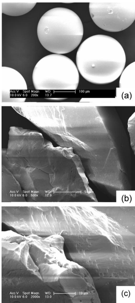
**FIGURE 6. ESEM images of (a) spherical glass bead collectors (200× magnification, 100 μm bar) and irregularly shaped quartz grains at (b) 500× magnification (50 μm bar) and (c) 2000× magnification (10 μm bar).**
