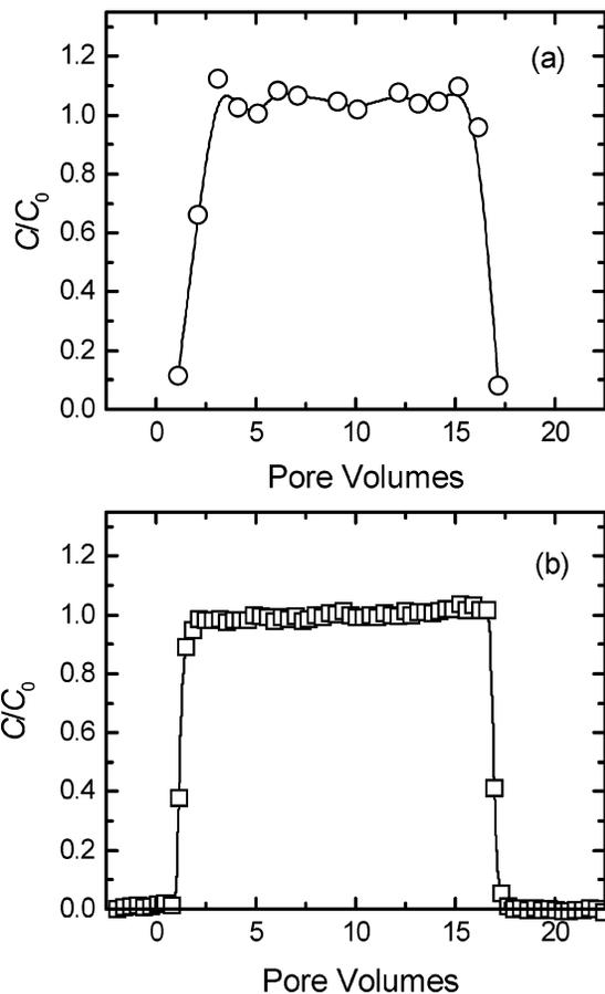
**FIGURE 7.** Breakthrough curves for experiments conducted in columns packed with soda-lime glass beads with (a) *C. parvum* oocysts and (b) 4.1  $\mu\text{m}$  model latex particles suspended in DI water. Other experimental conditions were as follows: approach velocity = 0.042 cm/s, porosity = 0.36, mean bead diameter = 0.23 mm, unadjusted pH (varied between 5.6 and 7.1), and temperature = 22–23 °C.
