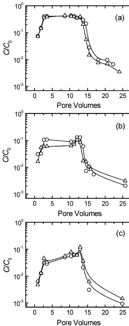
**FIGURE 2.** Breakthrough curves for two replicate experiments conducted with *C. parvum* oocysts in columns packed with clean quartz grains at three different solution ionic strengths: (a) 1 mM KCl; (b) 3.16 mM KCl; and (c) 10 mM KCl. Other experimental conditions were as follows: approach velocity = 0.042 cm/s, porosity = 0.43, mean grain diameter = 0.21 mm, pH 5.6–5.8, and temperature = 22–23 °C.
