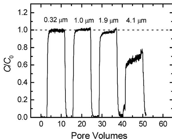
**FIGURE 8.** Breakthrough curves for experiments conducted with model latex particles of increasing diameter (0.32, 1.0, 1.9, and 4.1  $\mu\text{m}$ ) suspended in DI water in a column packed with clean quartz sand. Other experimental conditions include approach velocity = 0.042 cm/s, porosity = 0.43, mean grain diameter = 0.21 mm, pH 5.6–5.8, and temperature = 22–23 °C.
