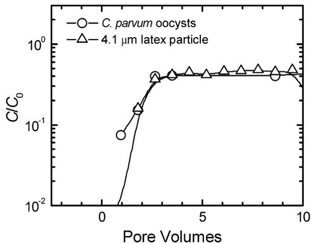
**FIGURE 4.** Breakthrough curves for experiments conducted with *C. parvum* oocysts and 4.1  $\mu m$  model latex particles in columns packed with clean quartz sand at 1 mM ionic strength. Other experimental conditions include approach velocity = 0.042 cm/s, porosity = 0.43, mean grain diameter = 0.21 mm, pH 5.6–5.8, and temperature = 22–23  $^{\circ}C$ .
