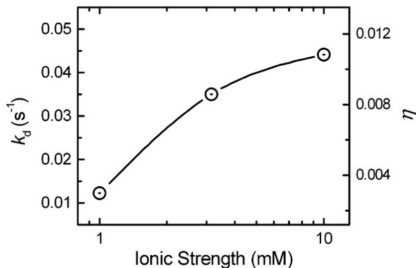
**FIGURE 3.** Influence of ionic strength on the *C. parvum* oocyst deposition rate coefficient ( $k_d$ ) and the corresponding single-collector removal efficiency ( $\eta$ ) in a column packed with quartz sand. Each data point represents the average value determined from all experiments conducted at a given ionic strength. Oocyst deposition rate coefficients were calculated using breakthrough concentrations ( $C/C_0$ ) in Figure 2 and eq 1.
