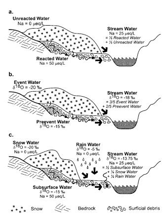
**Figure 3.** Schematic diagrams depicting information provided by hydrograph separations: (a) two-component model using a chemical tracer; (b) two-component model using an isotopic tracer; and (c) three-component model using dual chemical and isotopic tracers.
