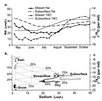
**Figure 9.** Fern Creek sensitivity analysis with varying subsurface component sodium concentrations and  $\delta^{18}$ O values: (a) model inputs and (b) mixing diagram.
