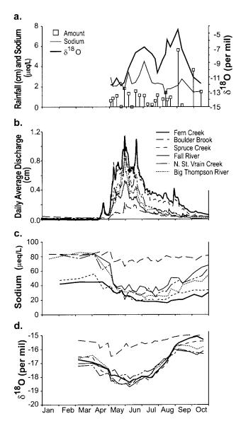
**Figure 2.** January through October 1994: (a) elevationally averaged rain amount, sodium concentration, and  $\delta^{18}$ O; (b) area-normalized daily average discharge; (c) stream water sodium concentrations; and (d) stream water  $\delta^{18}$ O composition.
