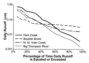
**Figure 8.** Flow-duration curves. Slopes of the Spruce Creek and Fall River flow-duration curves are similar to Fern Creek and Big Thompson River slopes.
