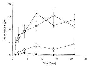
FIGURE 2. Kinetics of dissolution of cinnabar (2 g/L) by F1 hydrophobic acid at concentrations of 5 mg C/L ( $\bullet$ ), 20 mg C/L ( $\bigcirc$ ), 50 mg C/L ( $\bigtriangledown$ ), and 100 mg C/L ( $\bigtriangledown$ ). Error bars represent standard deviation from triplicate analysis.
