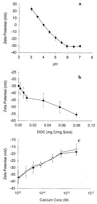
FIGURE 4. Results of electrophoretic mobility measurements ( $\zeta$ -potential) on cinnabar surfaces. (a) pH titration of cinnabar to determine pH<sub>pzc</sub>. (b) Change in  $\zeta$ -potential as a function of organic matter (F1-HPoA) concentration. (c) Change in  $\zeta$ -potential as a function of calcium concentration in the absence of organic matter ( $\bullet$ ) and in the presence of F1-HPoA at 0.05 mg C/mg cinnabar ( $\bigcirc$ ).
