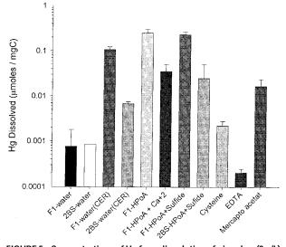
FIGURE 5. Concentrations of Hg from dissolution of cinnabar (2 g/L) by unfractionated organic matter in water samples (CER: samples passed through cation-exchange resins) from Florida Everglades, by model ligands, and in the presence of calcium and sulfide (see text for concentrations used). Error bars represent standard deviation from triplicate analysis.
