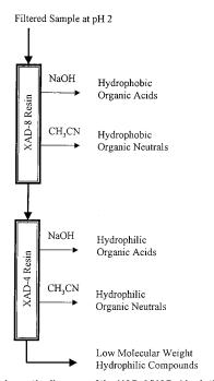
FIGURE 1. Schematic diagram of the XAD-8/XAD-4 isolation scheme.
