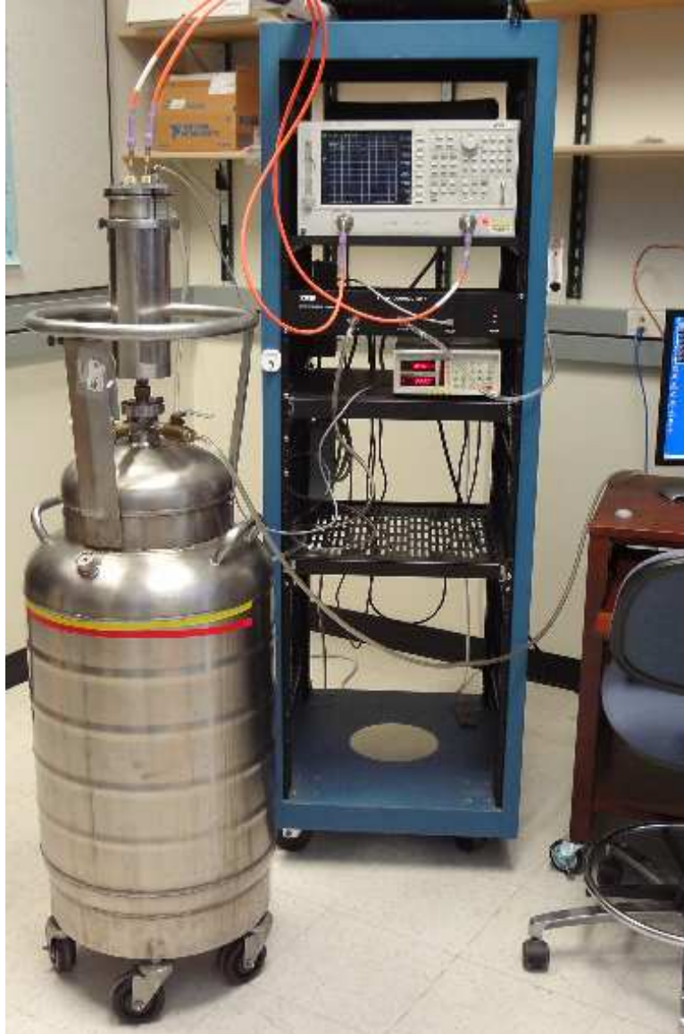
Figure 3.3: A photograph of the measurement setup, showing the flow-type cryostat on top of a liquid helium filled dewar. To the right of the dewar are the network analyzer, flow control unit, and temperature controller, shown from top down.
