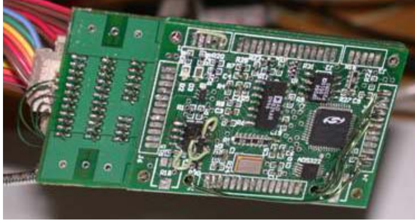
Figure 53 – Photograph of the CSAC control electronics board. This board was placed on the back side of the integrated LO-PP physics board.
