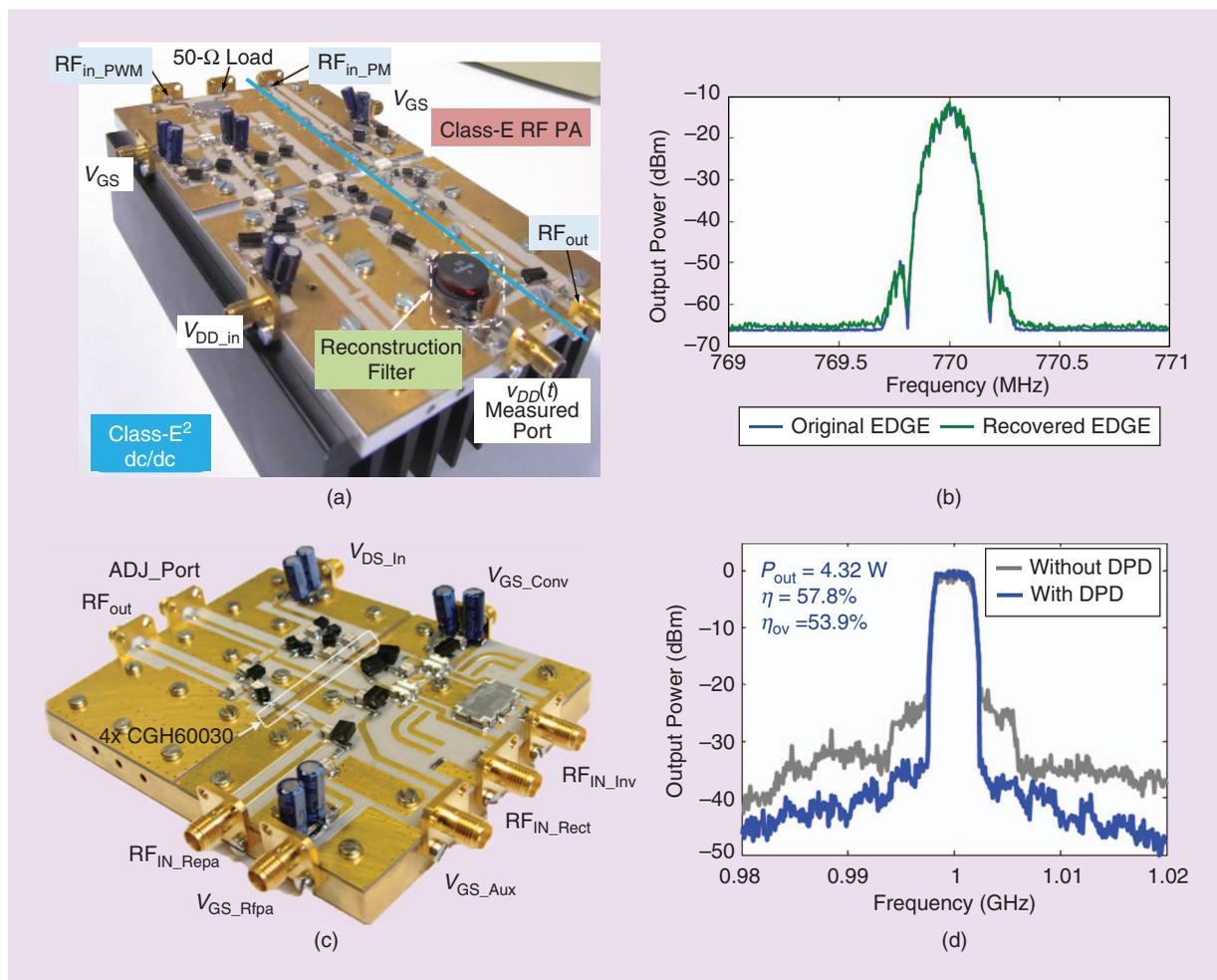
**Figure 13.** Polar transmitter implementations integrating class-E<sup>2</sup> resonant converters: (a) a packaged device version at 770 MHz (from [19]) and (b) the reproduced EDGE signal spectrum. (c) A die-based architecture at 1 GHz producing a one-carrier WCDMA signal, as shown in (d). DPD: digital predistortion.
