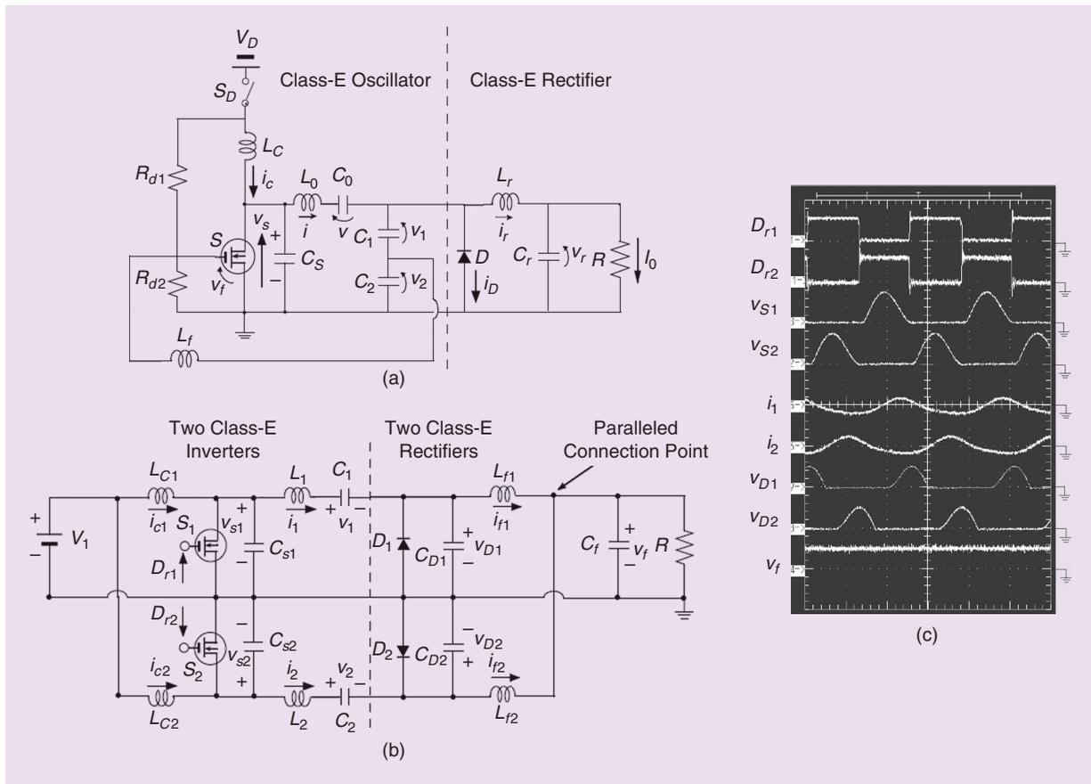
**Figure 5.** The circuit topologies of class-E<sup>2</sup> converters as designed by Chiba University researchers: (a) a 1.55-W converter with oscillating inverter at 2 MHz (from [20]) and (b) a 3.2-W interleaved converter operating at 1 MHz (from [21]). (c) Experimental waveforms for the converter in Figure 5(b) (also from [21]).
