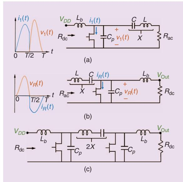
**Figure 4.** (a) The class-E inverter, or PA, and (b) its transistor-based time-reversed dual, a class-E synchronous rectifier. (c) A basic class-E<sup>2</sup> dc-to-dc converter obtained when cascading (a) and (b). For operation at RF/microwave frequencies, the parallel capacitance ( $C_p$ ) is generally provided by the device output capacitance ( $C_{out}$ ). Characteristic waveforms for the switch voltage and current are also shown in (a) and (b).
