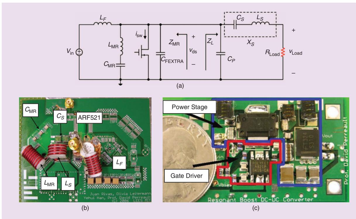
**Figure 2.** (a) The schematic and (b) a photo of the 30-MHz class- $\Phi_2$  inverter in [11], based on the ARF521 MOSFET from Microsemi. (c) A photo of a complete 110-MHz class- $\Phi_2$  boost converter, with the output voltage control circuitry placed on the other side of the printed circuit board [12]. (Images courtesy of Dave Perreault, Massachusetts Institute of Technology.)
