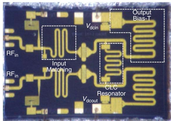
**Figure 12.** A fully integrated class-E<sup>2</sup> synchronous dc-to-dc converter at 4.6 GHz [35]. The 3.8-mm × 2.3-mm GaN-on-SiC die using the Qorvo 150-nm gate process demonstrates a total efficiency above 50% with no external components. CLC: capacitor-inductance-capacitor.
