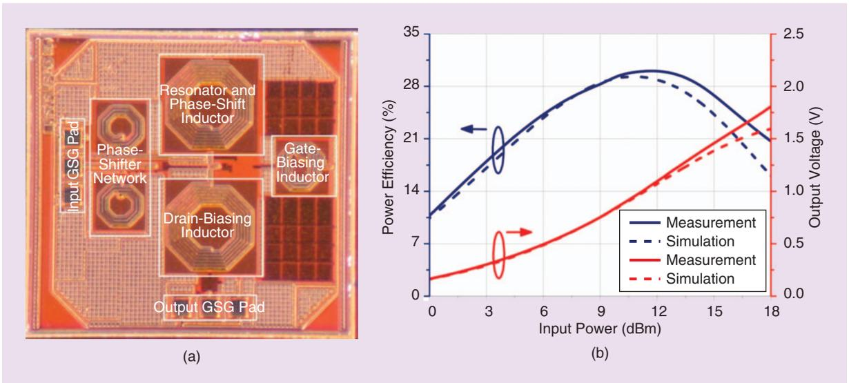
**Figure 6.** (a) The class-E synchronous rectifier in [24]. (b) The power efficiency and output voltage as a function of available power at a 250-Ω load. (Images courtesy of Thomas Johnson, University of British Columbia.) GSG: ground-signal-ground.
