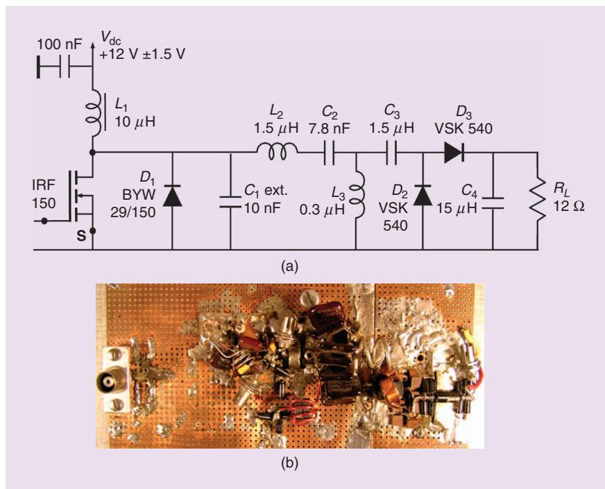
**Figure 1.** (a) A schematic of the experimental converter in [4] (driver not included) and (b) a photo of the 100-W, 14-MHz converter in [6]. (Photo courtesy of Richard Redl.)
