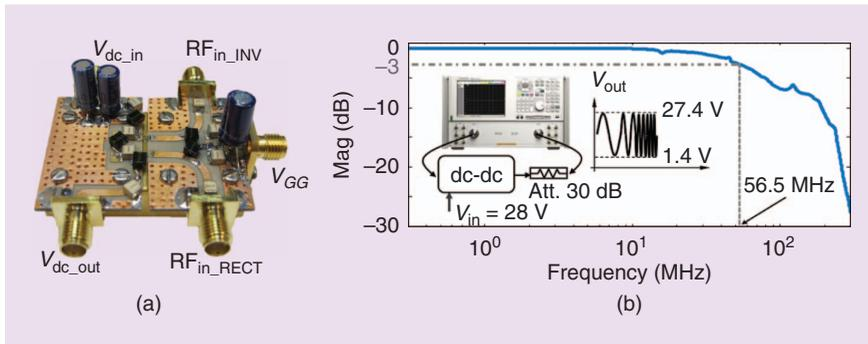
**Figure 10.** A die-based GaN high electron-mobility transistor (HEMT) class- $E^2$  converter at 1 GHz: (a) a photo of the implementation and (b) the measured dynamic performance.
