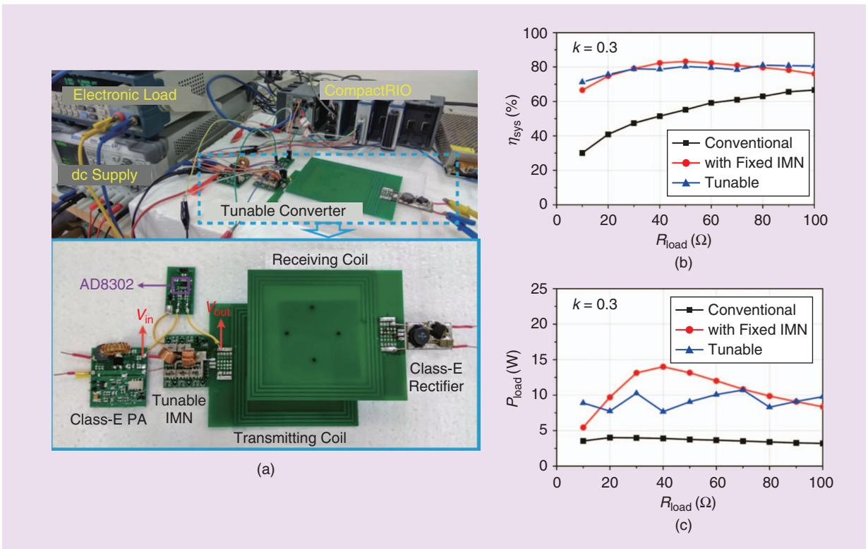
**Figure 7.** (a) A dynamically controlled class-E<sup>2</sup> dc-to-dc converter at 6.78 MHz for WPT [26]. A comparison of (b) efficiency and (c) output power performance versus dc load with  $k = 0.3$  for a conventional topology, a converter with a fixed-input matching network, and a tunable converter. CompactRIO: a real-time embedded industrial controller made by National Instruments; IMN: impedance matching network.
