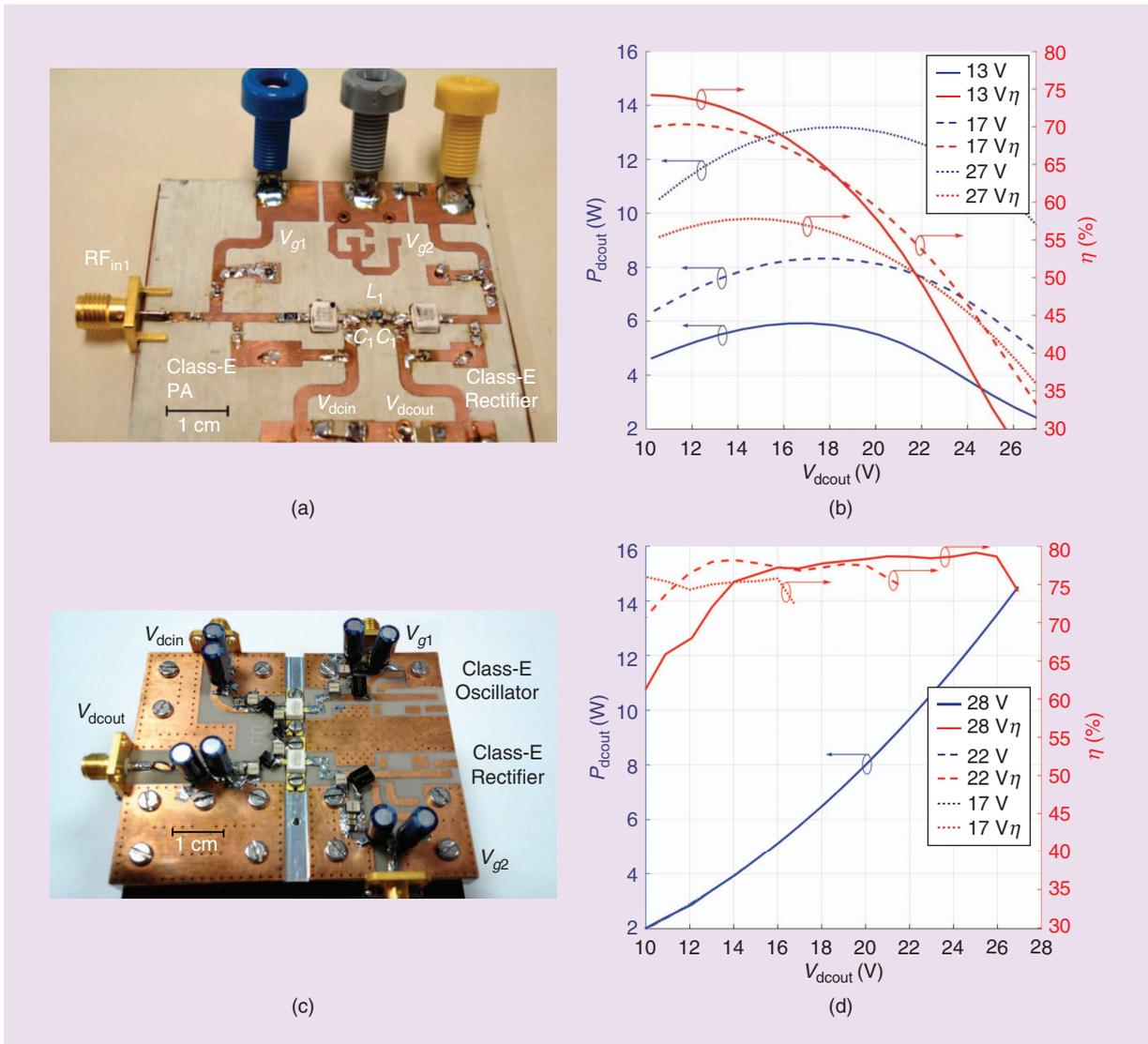
**Figure 11.** A class-E<sup>2</sup> self-synchronous converter at 1.2 GHz [23]: (a) a photo and (b) the measured output power and efficiency profiles with output dc voltage. A class-E<sup>2</sup> oscillating and self-synchronous converter at 1 GHz [23]: (c) a photo and (d) the measured output power and efficiency profiles with output dc voltage.
