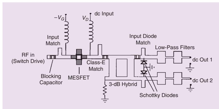
**Figure 3.** The layout of a class-E dc-dc converter, switching at 4.5 GHz [13]. The converter uses a class-E inverter (PA) with a GaAs MESFET and a balanced microwave Schottky diode rectifier. It achieves 64% efficiency for a 3-V dc input and an 87-Ω load.
