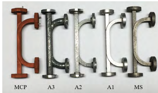
Figure 2.6: Photograph of WR-10 20-dB waveguide couplers implemented in a variety of materials. From left to right: metal (Cu) coated plastic (MCP), 3 AlSi10Mg with different laser settings, and maraging steel (MS).
