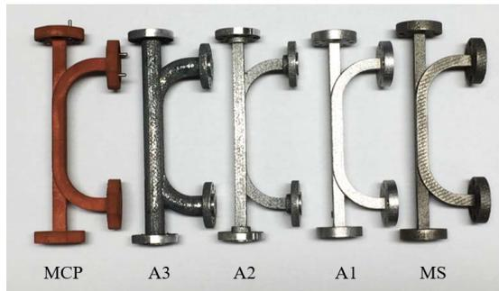
Fig. 2. Photograph of WR-10 20-dB waveguide couplers implemented in a variety of materials. From left to right: MCP, 3 AlSi10Mg with different laser settings, and MS.
