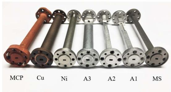
Fig. 1. Photograph of straight 10-cm WR-10 waveguides implemented in a variety of materials. From left to right: MCP, GRCoP-84 (Cu), Inconel 625 (Ni), 3 AlSi10Mg with different laser settings, and MS.
