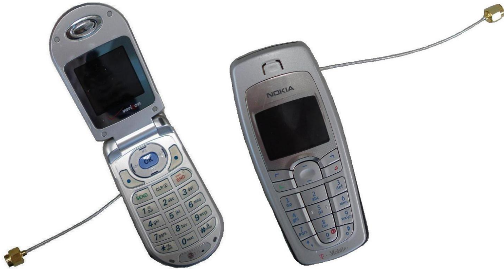
Figure 2.10: Sample cell phones operating around 800MHz and 1.9GHz cell uplink frequencies, with coaxial cable and SMA connector attached for antenna measurements. LG VX3200 phone is on the left; Nokia 6010 phone is on the right.
