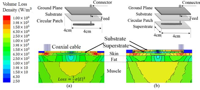
Fig. 2. Volume loss density of circular patch with and without superstrate are compared. (a) Patch is designed to maximize power deposition into the buried muscle layer. (b) Adding appropriate superstrate matches the probe to deeper tissue layers and doubles the power transfer to the muscle layer.
