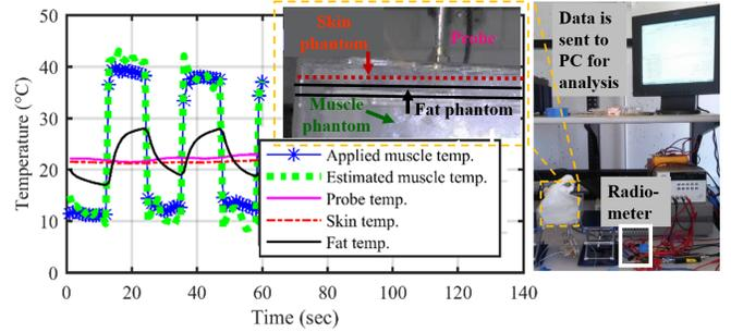
Fig. 5. Measured radiometric temperature of the muscle phantom (green) tracks the actual temperature (blue). Probe and skin (red) and fat (black) temperatures change at a much longer time scale.
