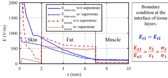
Fig. 3. Simulated  $E_{tang}$  and  $E_{norm}$  in different tissue layers with an without probe superstrate. The skin surface is at  $z=0$ .
