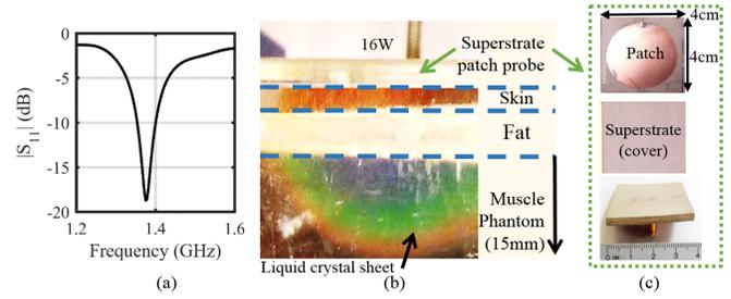
Fig. 4. (a) Measured  $S_{11}$  of the probe on skin, fat, and muscle phantom. (b) Temperature profile of superstrate patch measured with a liquid crystal sheet placed in the transparent muscle phantom under the transmitting patch. A ZHL-15W-43 power amplifier is used for 60 s to heat up the tissue phantoms. (c) fabricated superstrate patch probe.
