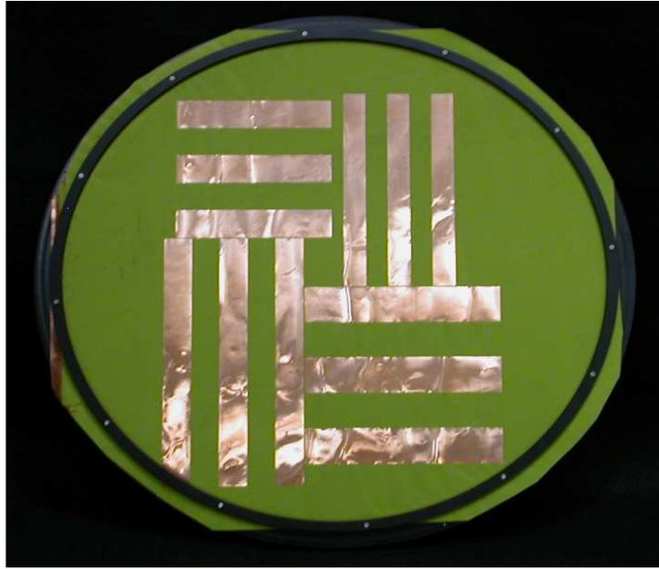
Figure 5.6: Resolution target used as concealed object in linear array images. The bars are made of copper tape and vary in size from 10 mm up to 20 mm.
