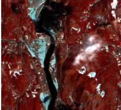
Figure B.1: Sample of image acquired by Hyperion sensor. This sensor offers up to 220+ contiguous spectral bands measuring from 0.4 $\mu\text{m}$  to 2.5 $\mu\text{m}$ . It acquires visible/near-infrared (400 nm to 1000nm) and shortwave infrared (900 nm to 2500 nm) spectral data. The spatial resolution is 30 meters and each image covers a 7.5 km x 100 km area
