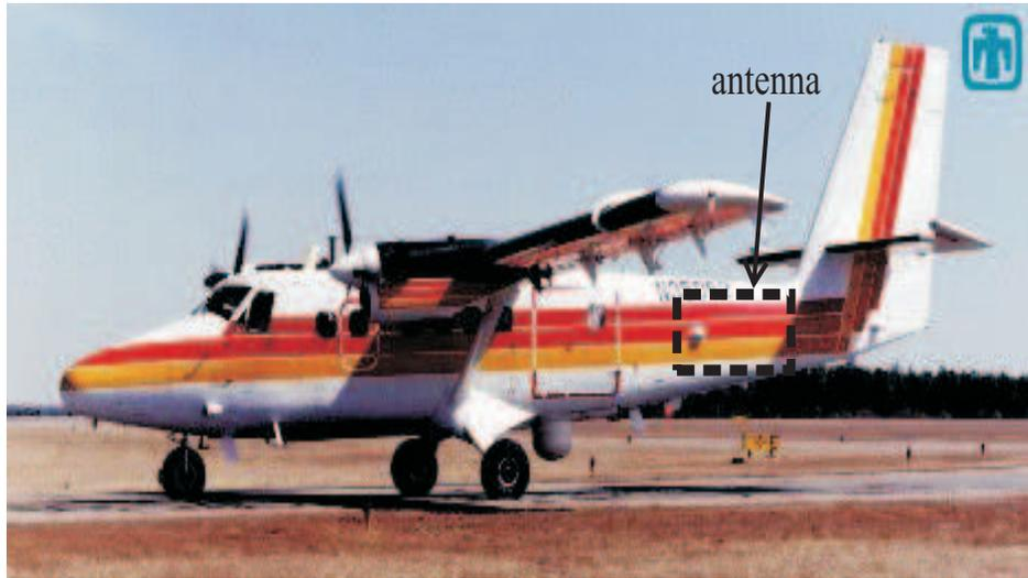
Figure 2.1: Sandia National Laboratory SAR platform aircraft carrying a complete data collection system including radar, GPS-aided IMU, fully gimballed antenna, real-time image formation processor, high capacity data storage system, and optionally a real-time automatic target recognition processor. Photograph used with permission from Sandia National Laboratory.
