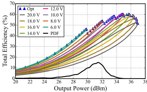
Fig. 8. Compilation of measured phase sweeps for swept supply levels from 6 V to 20 V in 2 V increments at 9.7 GHz. The optimal trajectory is selected to maximize  $\eta_{tot}$ . In black is the PDF of a 6 dB PAPR QPSK signal used to calculate average total efficiency.
