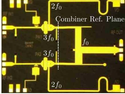
Fig. 2. Photograph of ML-CO GaN MMIC PA, showing harmonic terminations and combiner design reference plane. The internal PAs operate in Class-F, with the combiner providing all fundamental frequency matching. Overall size is  $3.8\text{ mm} \times 3.2\text{ mm}$ .
