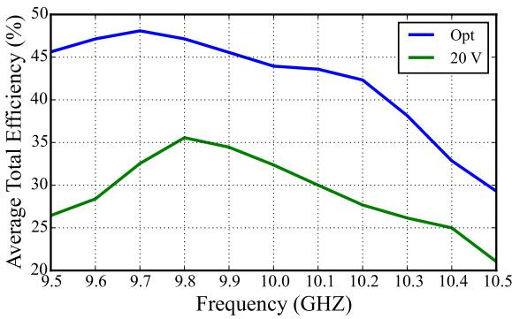
Fig. 9. Comparison of average total efficiency across frequency between the optimal trajectory and 20 V supply, showing improvements between 8 and 19 points. Optimal operation achieves 400 MHz of bandwidth with  $\eta_{tot,avg} > 45\%$ .
