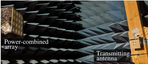
Fig. 6. Photograph showing test setup for measuring rectenna arrays. An RF power source, variable dc load, and voltmeter are kept outside of the anechoic chamber.
