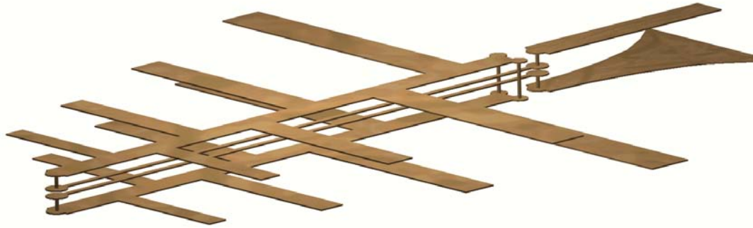
Figure 3.9: A drawing of the printed log periodic dipole antenna
