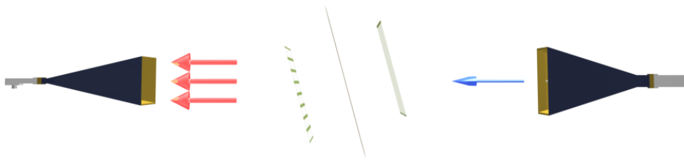
Figure 4.13: Gain measurement setup shown from above for the active-antenna array operating in resonant mode.
