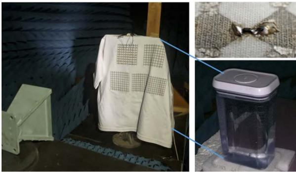
Fig. 18. Photograph of tee-shirt on phantom in the anechoic chamber during measurements, with the phantom shown on the bottom right. A detail of a fabricated single array element is shown on the top right.
