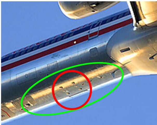
Fig. 1. Typical location of the altimeter radar on a commercial aircraft, the red circle shows the location of the altimeter antennas and the green oval is the approximate region where the harvesters can be located.
