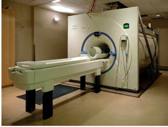
Figure 3.2: Image of the passively shielded 7 T Siemens MRI scanner at the Center for Magnetic Resonance Research.
