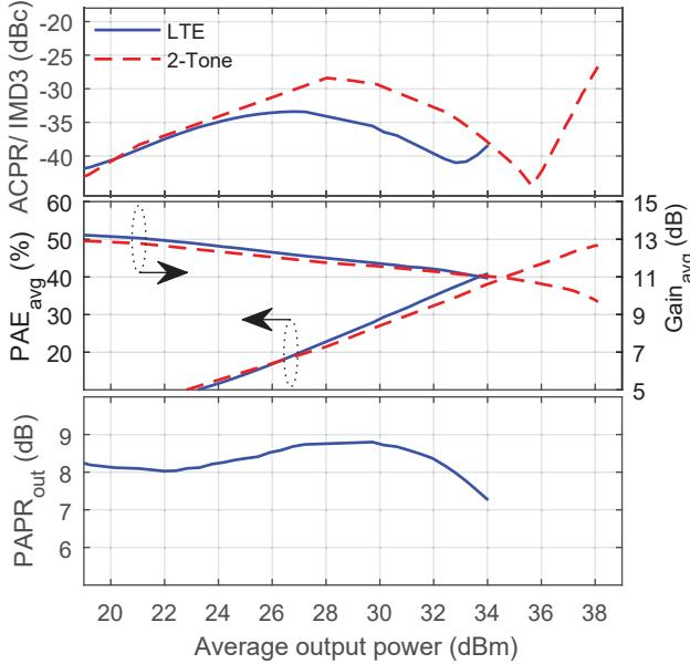
Fig. 2. ACPR/IMD3, average PAE and gain, and output PAPR vs. average output power for a 5-MHz 8.5-dB PAPR LTE signal and for a 5-MHz spaced two-tone for the DPA at 3.5 GHz.
