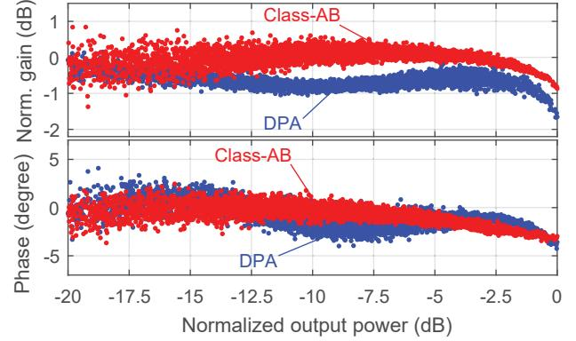
Fig. 5. AM-AM and AM-PM for the DPA and the class-AB PA for a LTE signal summarized in Fig. 4.
