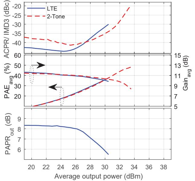
Fig. 3. ACPR/IMD3, average PAE and gain, and output PAPR vs. average output power for a 5-MHz 8.5-dB PAPR LTE signal and for a 5-MHz spaced two-tone for the class-AB PA at 3 GHz.
