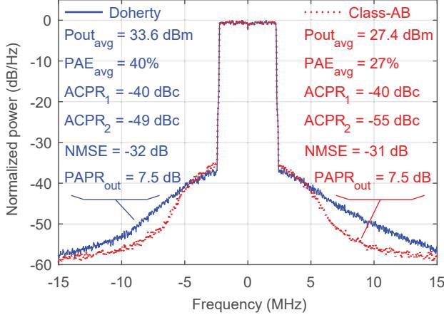
Fig. 4. Normalized power spectral density for a 5-MHz 8.5-dB PAPR LTE signal at 3.5 GHz for the DPA and at 3 GHz for the class-AB PA.
