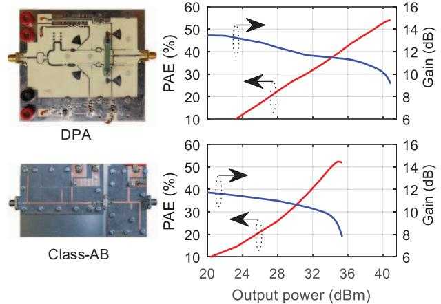
Fig. 1. Photograph of the DPA and the class-AB PA used for the comparison (left) and CW performance after post-optimized biases and supplies (right).
