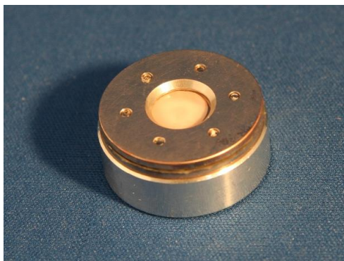
Fig. 3. Copper holder with an uncoated nanopore polycarbonate membrane mounted in it.
