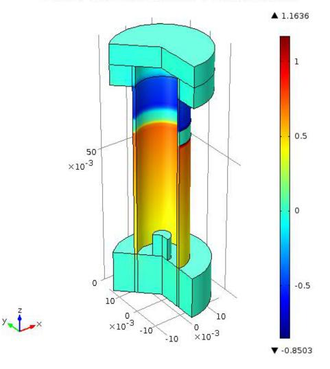
Surface: Temperature gradient, z component (K/m)
