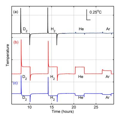
**Figure 3.** Experimentally observed temperature changes due to gas loading of Pd-impregnated alumina (a) in the absence of an artificially produced thermal gradient; (b) in the presence of a hot spot; (c) in the presence of a cold spot. Pressurizations were carried out with deuterium, hydrogen, helium and argon.
