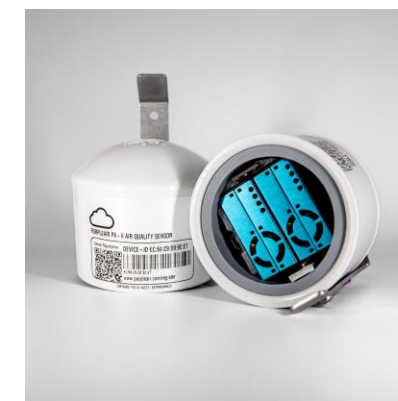
Figure 3: Classic PurpleAir PA-II particulate sensor which was placed on the outside of the 25 homes
