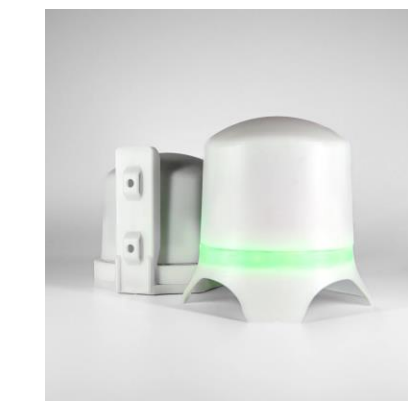
Figure 4: PurpleAir Zen model particulate sensor which was placed on the inside of the 25 homes
