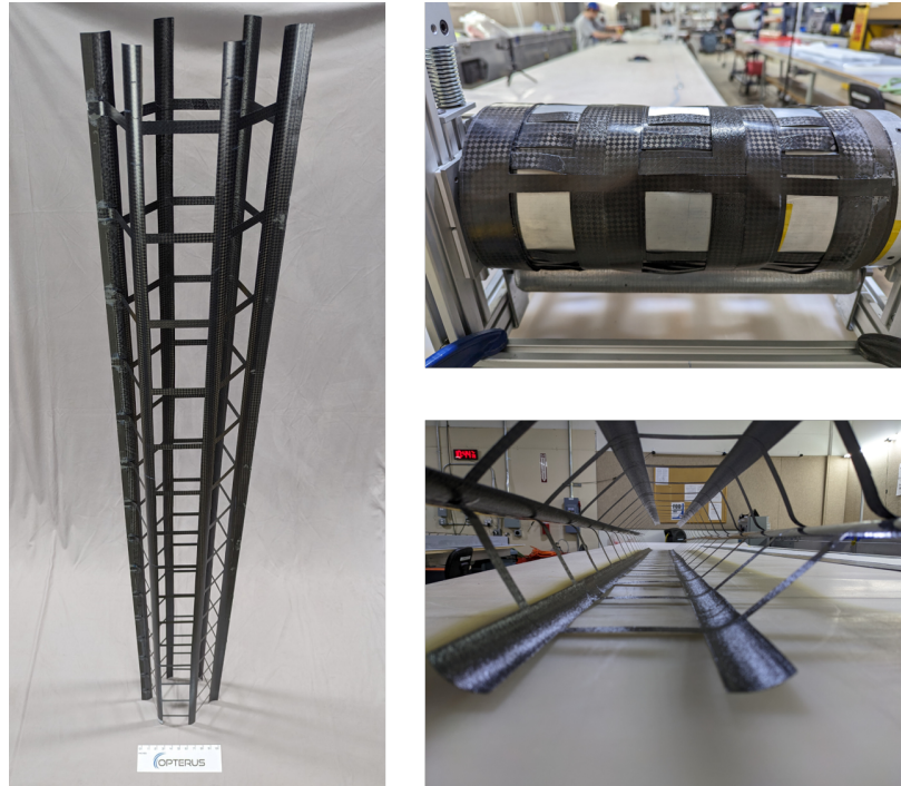
Fig. 1 The Phase I SSTM boom in deployed and rolled configurations.
