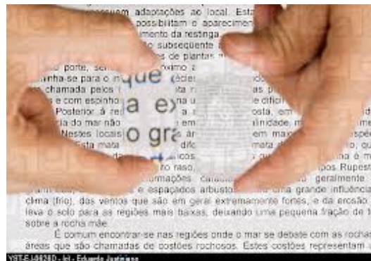
converging lens “bi-convex” has two convex surfaces
