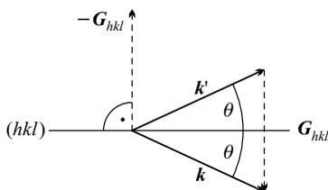
**Fig. 8.4.** Geometry of the wave vectors of the incident and scattered beams, the reciprocal-lattice vector satisfying the Laue condition, and the crystal plane perpendicular to it
