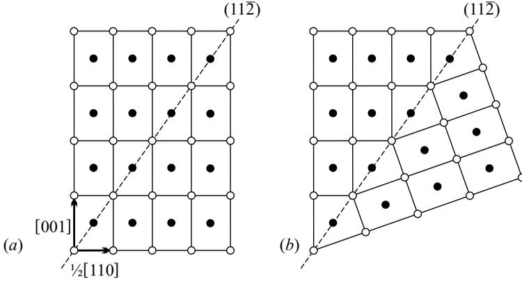
**Fig. 9.26.** (a) Atomic arrangement in a face-centered cubic crystal in the plane perpendicular to the direction  $[1\bar{1}0]$ . (b) Atomic arrangement in a twin crystal with a twin boundary at a  $(11\bar{2})$  plane. Atoms in the  $(1\bar{1}0)$  plane through the origin are marked by empty circles; atoms in front of and behind this plane are marked by full circles
