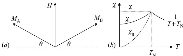
**Fig. 14.14.** (a) The orientation of the sublattice-magnetization vectors of an isotropic antiferromagnet in a magnetic field. (b) The temperature dependence of susceptibility
