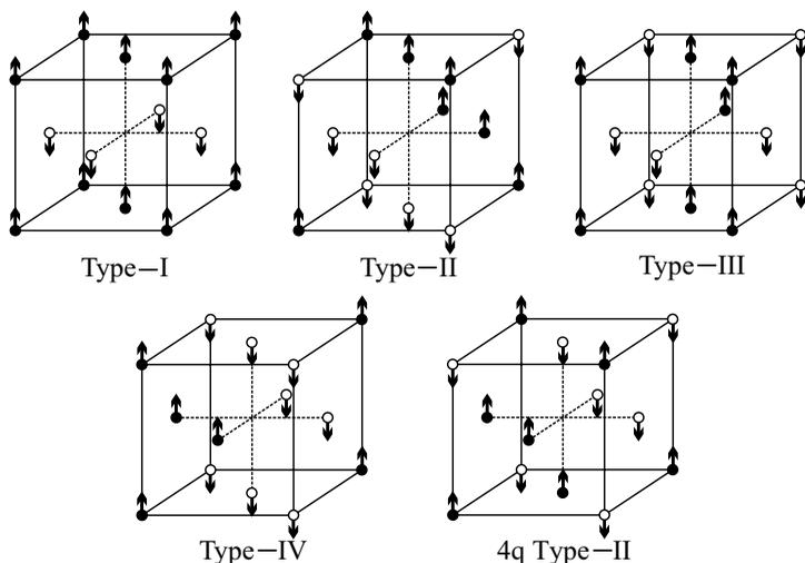
Fig. 14.4. Collinear magnetic structures in face-centered cubic crystals
