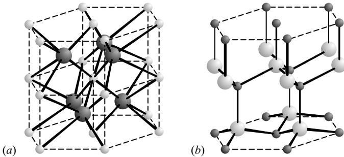
**Fig. 7.22.** Hexagonal crystal structures: (a) NiAs (B8) structure; (b) wurtzite (B4) structure
