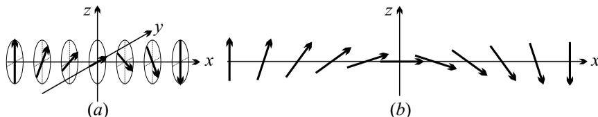
**Fig. 14.19.** Rotation of the magnetic moment for domain walls in the  $(y, z)$  plane: (a) Bloch wall; (b) Néel wall
