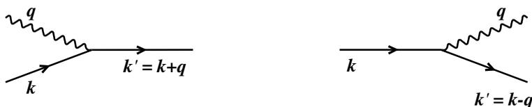
**Fig. 6.6.** Diagrammatic representation of the emission and absorption of quanta of lattice vibrations by electrons. Solid lines are electrons, wavy lines are lattice vibrations
