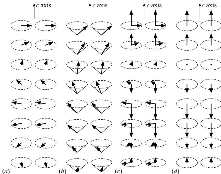
**Fig. 14.6.** Noncollinear magnetic structures in rare-earth metals: (a) the helical structure of dysprosium and holmium; (b) the conical ferromagnetic structure of holmium and erbium; (c) the sinusoidally modulated conical structure of erbium; (d) the longitudinal-wave structure of erbium
