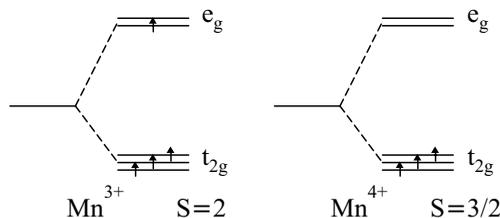
**Fig. 14.10.** The  $d$  electrons of  $\text{Mn}^{3+}$  and  $\text{Mn}^{4+}$  ions on the  $t_{2g}$  and  $e_g$  levels
