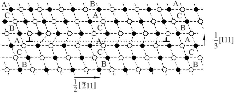
**Fig. 9.21.** Projection of a finite stacking fault bordered by partial dislocations in a face-centered cubic lattice on the  $(01\bar{1})$  plane. Atoms marked by empty circles lie in a  $(01\bar{1})$  plane, while those marked by full circles lie in the parallel plane in front or behind, separated by a quarter of the face diagonal  $[01\bar{1}]$
