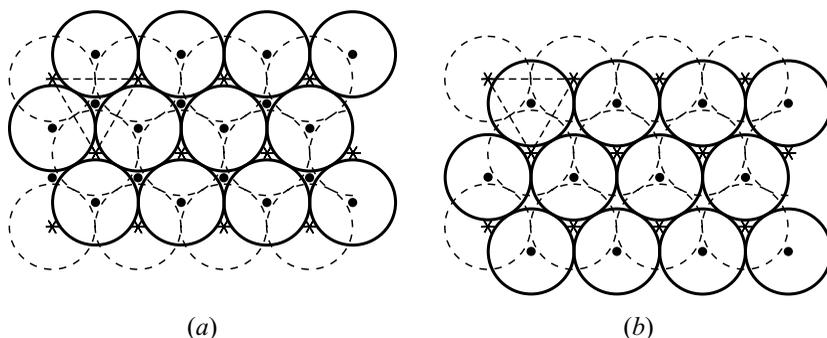
**Fig. 7.20.** Two possible ways of stacking hexagonal close-packed layers. Dashed-line circles (spheres) centered at asterisks (\*) mark the atoms of the lower layer. Relative to this layer (*A*), two arrangements – shown in (a) and (b) – are possible for the centers (●) of the spheres in the second layer. They are called type *B* and type *C* layers
