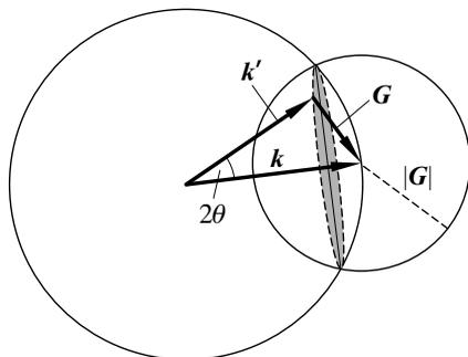
**Fig. 8.15.** The Ewald construction for the powder method
