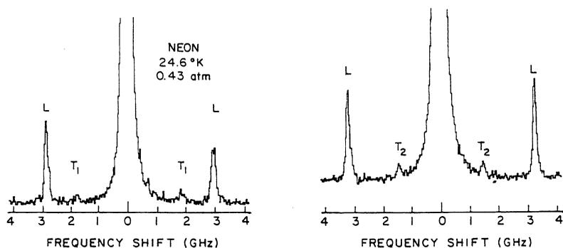
**Fig. 13.9.** Brillouin spectra of two single crystals of neon of different orientations, along a direction close to that of the direct beam [B. P. Stoichoff et al., *Proc. of the 2nd Int. Conf. on Light Scattering in Solids*, Paris, p. 450 (1971)]
