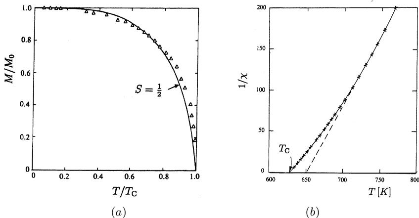
**Fig. 14.12.** Comparison of the measured magnetic properties of nickel [P. Weiss and R. Forrer, *Ann. de Phys.* **5**, 153 (1926)] with the results obtained in the mean-field theory for  $S = 1/2$ . (a) Magnetization and (b) inverse susceptibility, as functions of temperature
