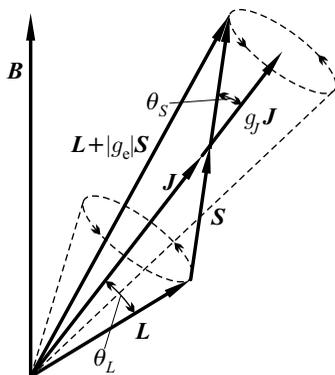
**Fig. 3.1.** Precession of the orbital angular momentum and the spin about the total angular momentum
