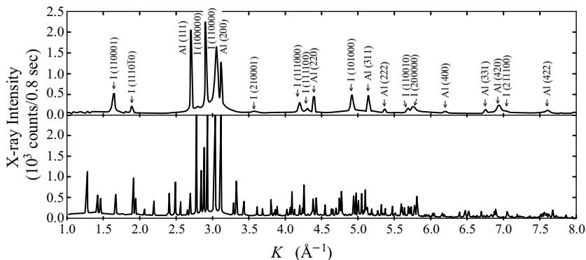
**Fig. 10.16.** High-resolution X-ray diffraction pattern of quenched (quasicrystalline) and annealed (crystalline) Al-Mn powder. Labels are Al and icosahedral Miller indices [P. A. Bancel et al., *Phys. Rev. Lett.* **54**, 2422 (1985)]
