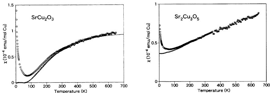
**Fig. 15.21.** Temperature dependence of the susceptibility of the two-leg ( $\text{SrCu}_2\text{O}_3$ ) and three-leg ( $\text{Sr}_2\text{Cu}_3\text{O}_5$ ) members of the series. Empty circles indicate raw data, while full circles are corrected data obtained by subtracting the Curie component [M. Azuma et al., *Phys. Rev. Lett.* **73**, 3463 (1994)]
