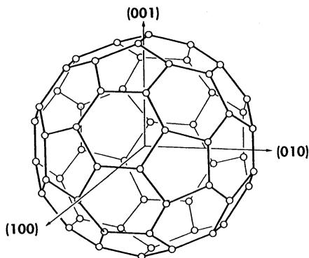
**Fig. 2.8.** The arrangement of carbon atoms in a  $\text{C}_{60}$  molecule
