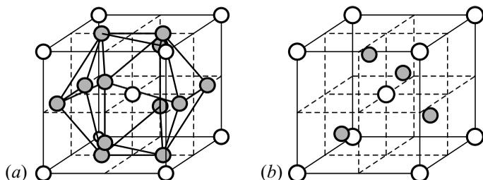
**Fig. 7.5.** Atomic arrangement in the primitive cell of compounds (a) of composition  $AB_3$  and structure A15; (b) of composition  $A_2B$  and structure C3
