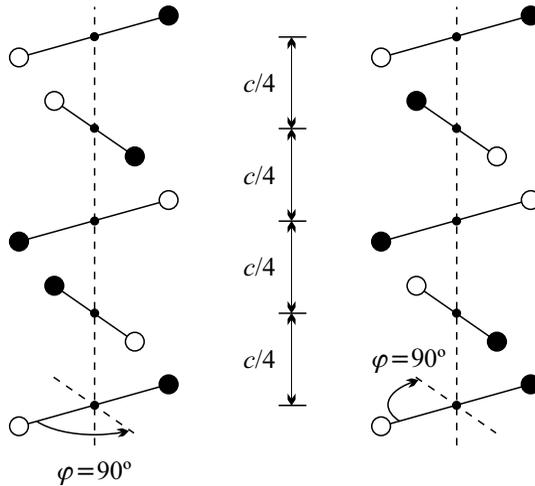
**Fig. 5.29.** Periodic structures with a fourfold screw axis. Rotation is clockwise in one case and counterclockwise in the other; both are followed by a translation of the crystal through one-quarter of the lattice constant
