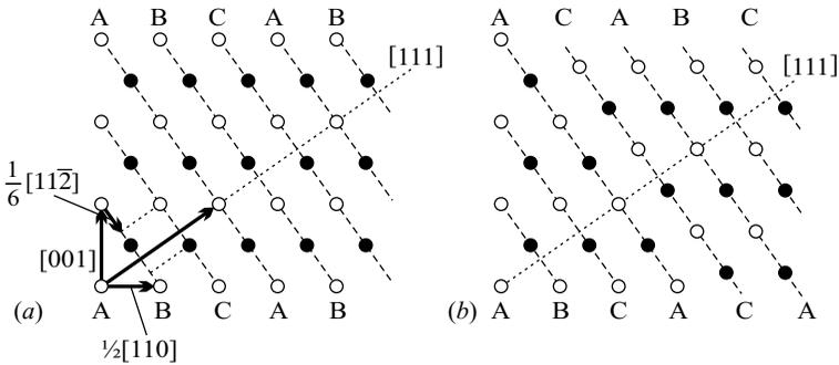
**Fig. 9.17.** Atoms in the  $(1\bar{1}0)$  plane through the origin and in the neighboring planes in a face-centered cubic lattice: (a) perfect crystal; (b) crystal with a stacking fault
