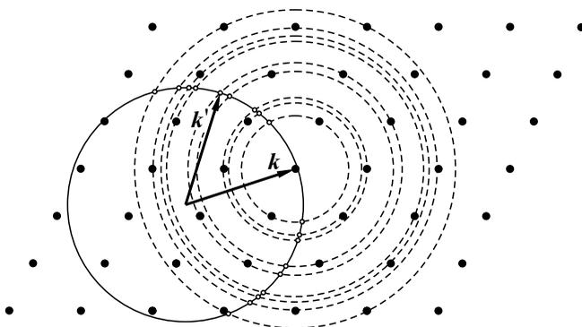
**Fig. 8.13.** The Ewald construction for a crystal rotating around an axis perpendicular to the direction of the incident beam. The solid circle is the section of the Ewald sphere, while dashed circles show the loci of the tips of reciprocal-lattice vectors when the sample is rotated
