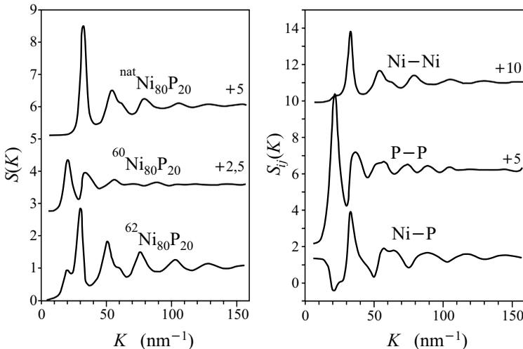
**Fig. 10.3.** Structure factors measured for various isotopic compositions of a two-component amorphous material,  $\text{Ni}_{80}\text{P}_{20}$ , and the derived partial structure factors. For better visibility, curves are shifted vertically. [P. Lamparter and S. Steeb, *Proc. of the Fifth Int. Conf. on Rapidly Quenched Metals*, p. 459 (1984)]
