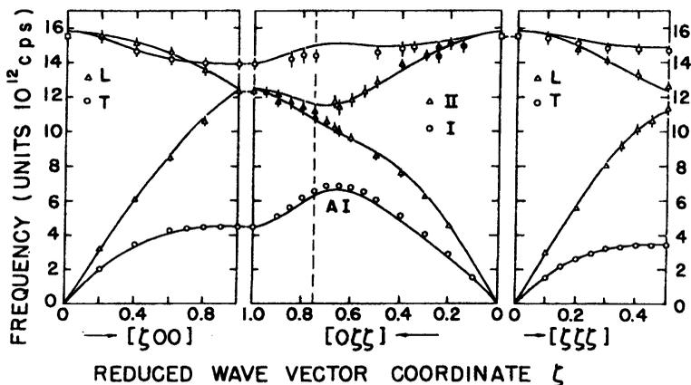
**Fig. 11.12.** Dispersion relations in some characteristic directions of the Brillouin zone for crystalline silicon, which contains two atoms per primitive cell. The solid line is a calculated curve fitted to experimental data. [G. Dolling, in *Inelastic Scattering of Neutrons in Solids and Liquids*, IAEA, Vienna, 1963, Vol. II., p. 37]
