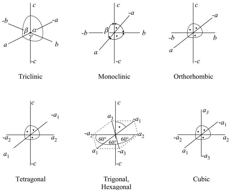
Fig. 5.17. Coordinate axes in the three-dimensional crystal systems
