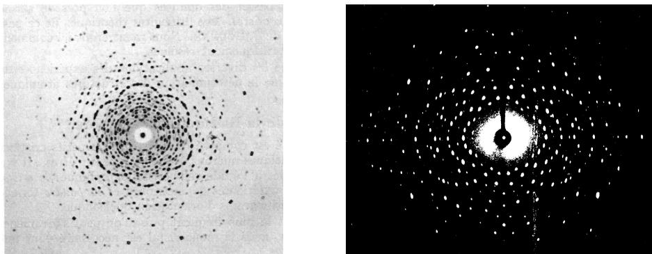
**Fig. 8.12.** Diffraction patterns along the direction of a crystallographic axis in beryllium and quartz obtained with the Laue method
