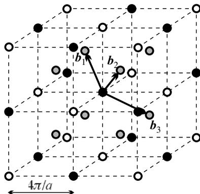
**Fig. 8.5.** Reciprocal-lattice vectors of the diamond structure that give rise to diffraction peaks of different intensities. The structure amplitude for vectors pointing to full circles, shaded circles, and empty circles are 2,  $1 \pm i$ , and 0. The intensity ratio of the corresponding Bragg peaks is therefore 4 : 2 : 0
