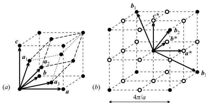
**Fig. 8.6.** (a) The primitive cell and the Bravais cell for a face-centered cubic crystal. (b) The body-centered cubic reciprocal lattice of the face-centered cubic direct lattice is indicated by full circles. The simple cubic lattice with the additional lattice points (empty circles) is the reciprocal of the lattice spanned by the primitive vectors  $\mathbf{a}$ ,  $\mathbf{b}$ ,  $\mathbf{c}$
