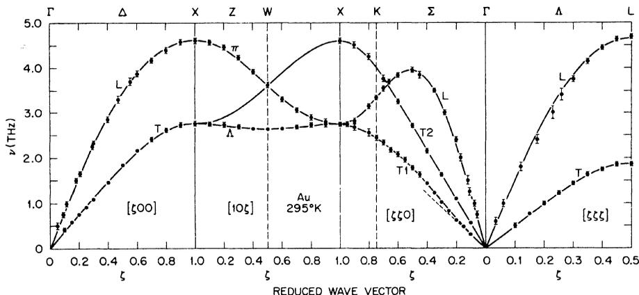
**Fig. 11.11.** Room-temperature dispersion relation of lattice vibrations for gold in the principal symmetry directions. The reduced wave vector  $\zeta = aq/2\pi$ . The solid curves were obtained from model calculations with several fitting parameters [J. W. Lynn et al., *Phys. Rev. B* **8**, 3493 (1973)]
