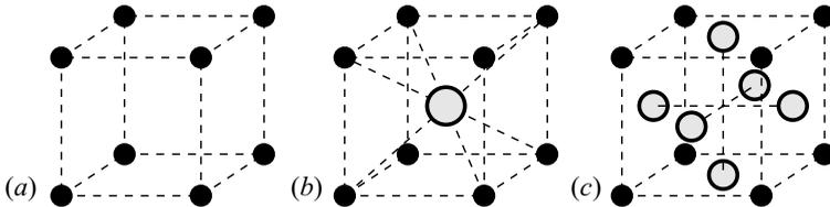
**Fig. 7.3.** Primitive cell for simple cubic structures with one-, two-, and four-point bases. (a) Monatomic cP1 ( $A_h$  or Po) structure; (b) diatomic cP2 (B2 or CsCl) structure; (c) tetratomic cP4 ( $L_{12}$  or  $Cu_3Au$ ) structure
