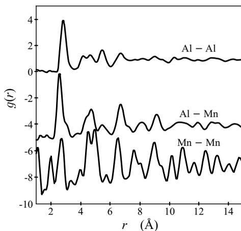
**Fig. 10.7.** Partial distribution functions for Al–Al, Al–Mn, and Mn–Mn in icosahedral quasicrystalline  $\text{Al}_{74}\text{Si}_5\text{Mn}_{21}$ , measured by M. de Boissieu et al. (*J. Phys.: Condens. Matter* **2**, 2499 (1990)) using neutron diffraction techniques. For better visibility, curves are shifted vertically
