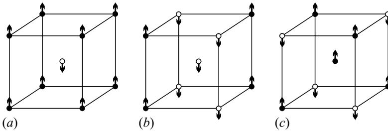
**Fig. 14.3.** Simple antiferromagnetic structures in body-centered cubic lattices
