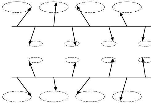
**Fig. 15.2.** Propagation of the two types of spin waves in a two-sublattice antiferromagnet
