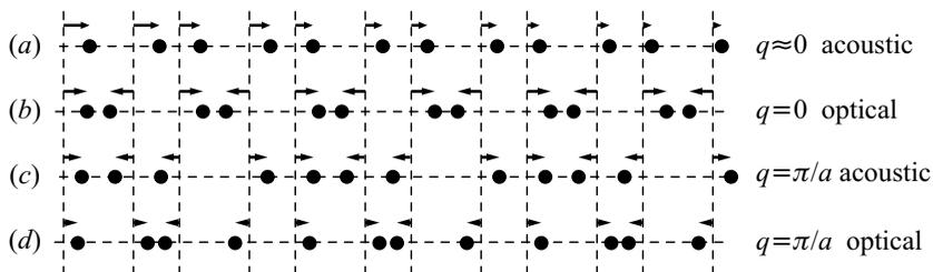
**Fig. 11.9.** Atomic displacements in the acoustic and optical modes of a dimerized linear chain in the long-wavelength limit for  $q = \pi/a$
