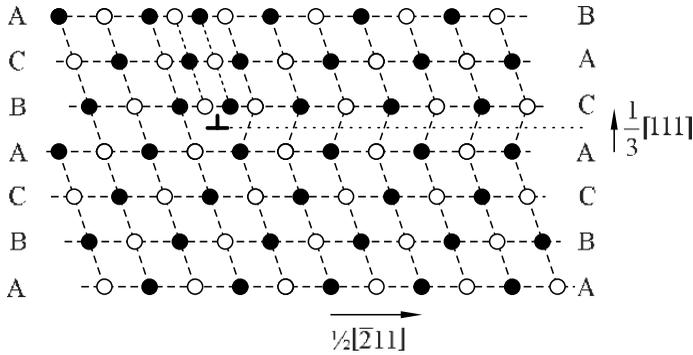
**Fig. 9.19.** Atomic arrangement around a Shockley partial dislocation. Atoms marked by empty circles lie in a  $(01\bar{1})$  plane, while those marked by full circles lie in the parallel plane in front or behind, separated by a quarter of the face diagonal  $[01\bar{1}]$
