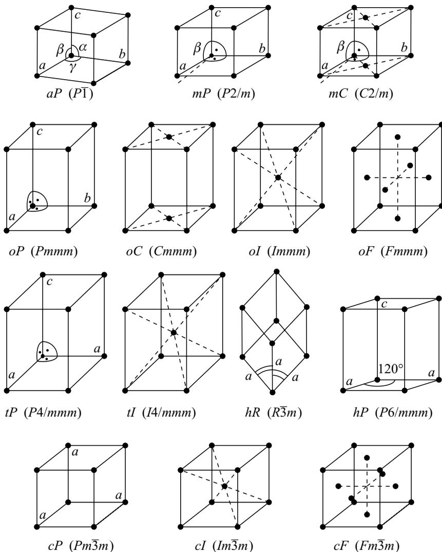
Fig. 5.23. The fourteen types of three-dimensional Bravais lattices
