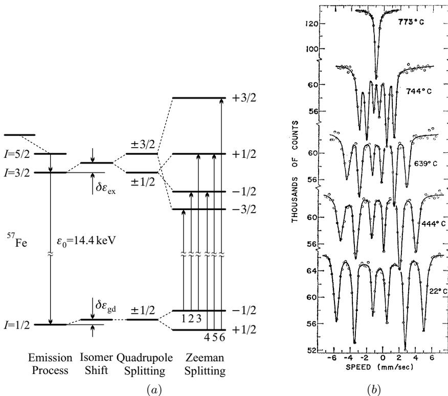
**Fig. 3.3.** (a) Splitting of the levels of  $^{57}\text{Fe}$  in the presence of a local magnetic field and a finite-gradient electric field. (b) Typical Mössbauer spectra for metallic  $^{57}\text{Fe}$  between room temperature and the Curie temperature [R. S. Preston, S. S. Hanna, and J. Heberle, *Phys. Rev.* **128**, 2207 (1962)]
