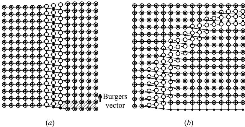
**Fig. 9.8.** Atomic positions above (large empty circles) and below (small full circles) the cut plane for (a) a screw dislocation; (b) a screw dislocation being transformed into an edge dislocation (mixed dislocation)
