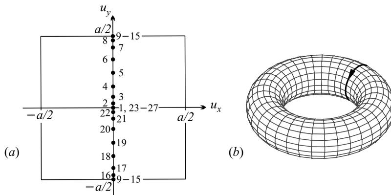
**Fig. 9.12.** (a) Displacement of the atoms around the Burgers circuit in Fig. 9.11 in the Wigner–Seitz cell of the lattice. (b) Mapping of the Burgers circuit into the torus in displacement space with periodic boundary conditions
