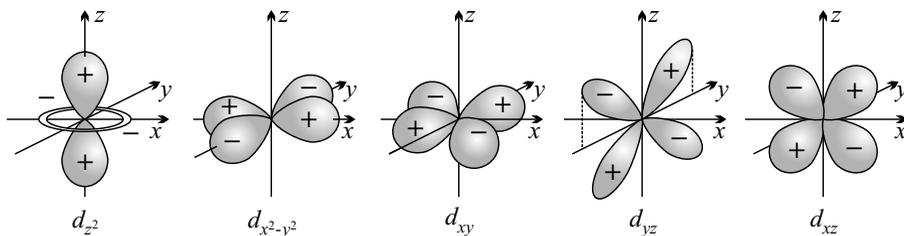
Fig. 6.1. Schematic representation of  $d$ -state wavefunctions
