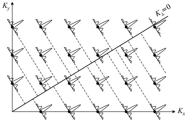
**Fig. 10.12.** Diffraction pattern of a finite strip of a square lattice and its section along the line  $K_{\perp} = 0$
