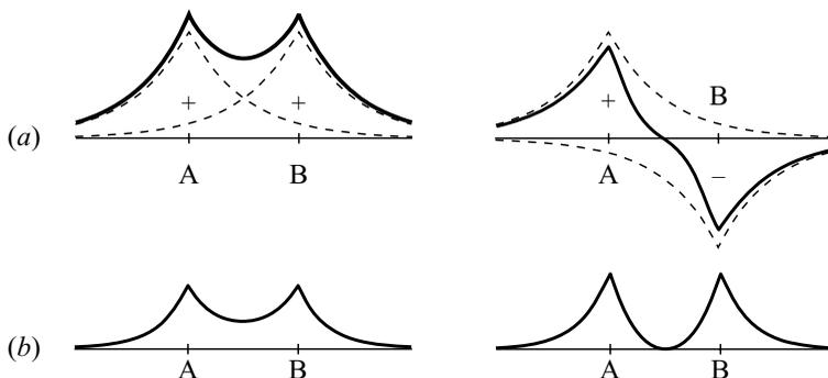
**Fig. 4.8.** (a) The wavefunction of the electrons for bonding (left) and antibonding (right) molecular orbitals in a two-atom system. (b) The corresponding charge distributions
