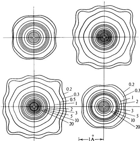
**Fig. 7.28.** Electron density in the (100) plane passing through atomic centers in a NaCl crystal, determined via the inverse Fourier transform of diffraction patterns [R. Brill, *Solid State Physics* **20**, 1 (1967)]
