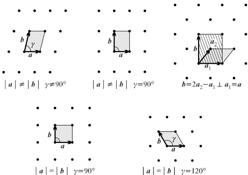
**Fig. 5.19.** Types of Bravais lattices and their primitive cells in two-dimensional crystal structures. The conventional unit cell (Bravais cell) is also indicated for the centered rectangular lattice
