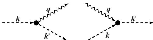
**Fig. 13.4.** Two types of Raman scattering. In Stokes processes a phonon is emitted; in anti-Stokes processes a phonon is absorbed
