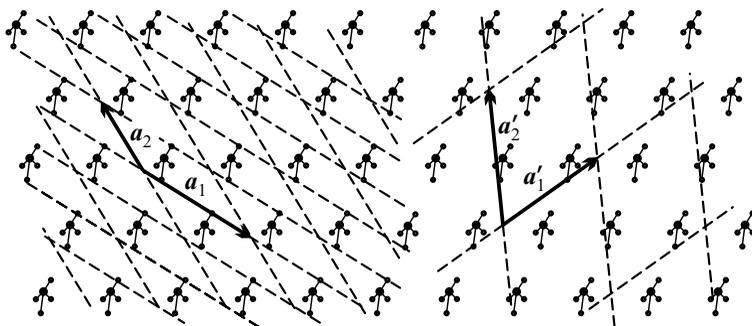
**Fig. 5.2.** A possible choice for the primitive vectors and a pair of new vectors obtained through their linear combination in a two-dimensional crystal
