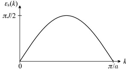
**Fig. 15.9.** Dispersion relation for spinons in an isotropic antiferromagnetic chain
