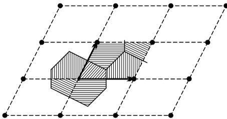
**Fig. 6.4.** Equivalence of the primitive cell spanned by the primitive vectors and the Brillouin zone of a two-dimensional reciprocal lattice. Regions with identical shading are displaced through some lattice vector
