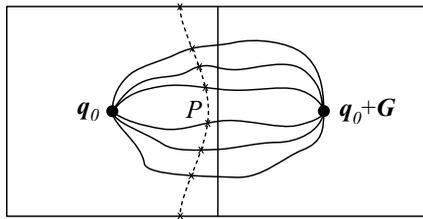
**Fig. 12.3.** Determination of the locus of the saddle point in the extended reciprocal space. Crosses ( $\times$ ) mark the maxima of the dispersion curve along the paths connecting  $\mathbf{q}_0$ , the center of the Brillouin zone, with an equivalent point  $\mathbf{q}_0 + \mathbf{G}$ . The minimum along the curve connecting these maxima is the saddle point  $P$
