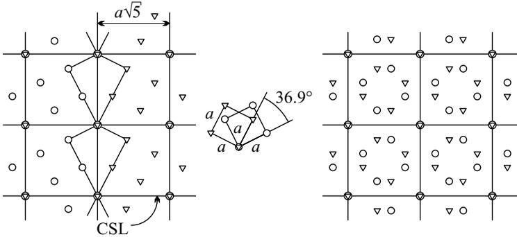
**Fig. 9.24.** The  $\Sigma 5$  coincident-site lattice of two grains in a cubic crystal tilted/twisted by  $36.9^\circ$ . The left side of the figure shows a tilt boundary, and the right one a twist boundary
