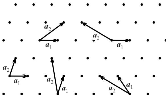
**Fig. 5.3.** Several possible choices for the pair of primitive vectors in a two-dimensional crystal. In each case every equivalent point can be reached by a integer linear combination of the primitive vectors
