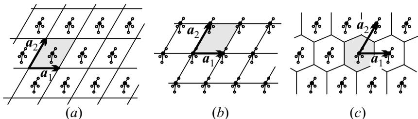
**Fig. 5.8.** Three different choices for the primitive cells (shaded areas) that allow for perfect tiling of the two-dimensional crystal. (a) and (b) differ only in the choice of the origin; (c) tessellation by Wigner-Seitz cells
