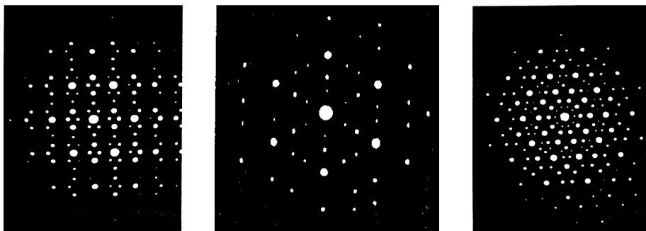
**Fig. 10.6.** Two-, three-, and fivefold symmetry in the electron diffraction patterns of quasicrystalline  $\text{Al}_{86}\text{Mn}_{14}$  [D. Shechtman et al., *Phys. Rev. Lett.* **53**, 1951 (1984)]
