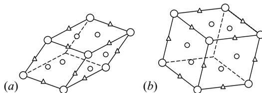
**Fig. 10.17.** (a) Thin and (b) thick rhombohedra used for the Penrose tiling of three-dimensional space. In quasicrystals atoms are located at marked positions, in vertices, on edges, or on face diagonals
