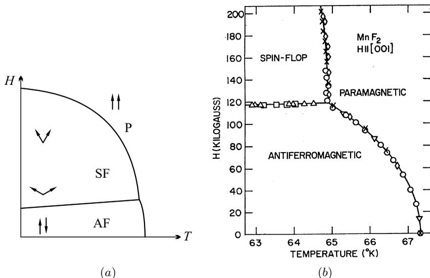
**Fig. 14.15.** The phase diagram (temperature vs. magnetic field plot) of an anisotropic antiferromagnet with an easy axis of magnetization. Part (a) shows a schematic phase diagram, while part (b) is the measured phase diagram of  $\text{MnF}_2$  below the Néel temperature [Y. Shapira and S. Foner, *Phys. Rev. B* **1**, 3083 (1970)]
