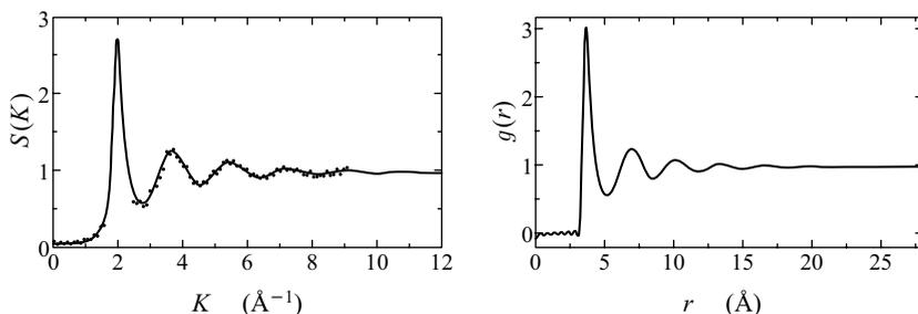
**Fig. 2.1.** The structure factor  $S(K)$  of liquid argon, measured at 85 kelvins in neutron scattering experiments, and the radial distribution function obtained from its Fourier transform [J. L. Yarnell et al., *Phys. Rev. A* **7**, 2130 (1973)]
