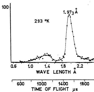
**Fig. 13.13.** The intensity of scattered neutrons as a function of energy for the one-phonon absorption peak in aluminum [K.-E. Larsson et al., *Proc. of the Symp. on Inelastic Scattering of Neutrons in Solids and Liquids*, Vienna, p. 587 (1960)]
