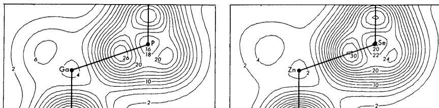
**Fig. 4.7.** Calculated density contours between two neighboring ions in a plane section of GaP and ZnSe crystals. [J. R. Chelikowsky and M. L. Cohen, *Phys. Rev. B* 14, 556 (1976)]
