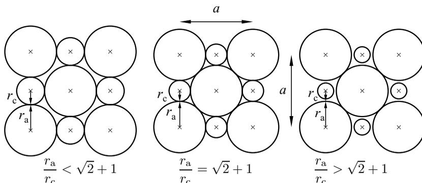
**Fig. 7.27.** Touching rigid spherical ions in the (110) plane of the sodium chloride structure, for various values of the anion–cation radius ratio
