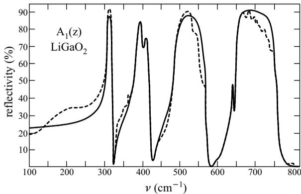
**Fig. 13.3.** Variations of the reflectivity of  $\text{LiGaO}_2$  in the infrared region. The dashed line represents measured data; the solid line is the result calculated from the frequencies of longitudinal and transverse optical phonons [P. Knoll and H. Kuzmany, *Phys. Rev. B* **29**, 2221 (1984)]
