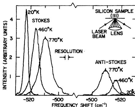
**Fig. 13.5.** Stokes and anti-Stokes components in the Raman spectrum of silicon at three different temperatures [T. R. Hart, R. L. Aggarwal and B. Lax, *Phys. Rev. B* **1**, 638 (1970)]
