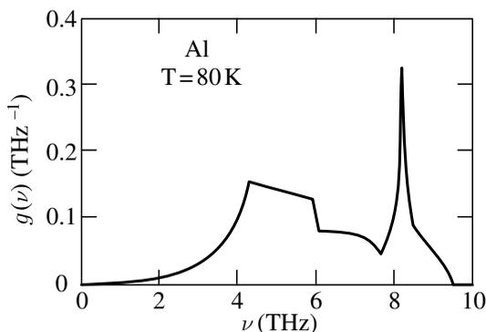
**Fig. 12.5.** Calculated phonon density of states in aluminum, with the characteristic Van Hove singularities [C. B. Walker, *Phys. Rev.* **103**, 547 (1956)]
