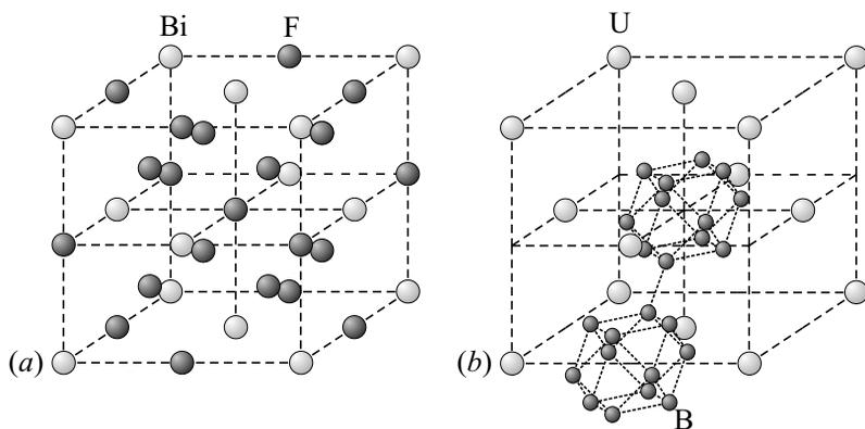
**Fig. 7.15.** Face-centered cubic structures: (a)  $\text{BiF}_3$  structure ( $\text{D0}_3$  structure), with 16 atoms per Bravais cell; (b)  $\text{UB}_{12}$  structure ( $\text{D2}_f$  structure) with 52 atoms per Bravais cell. Only two of the four cuboctahedra are shown; each contains twelve boron atoms
