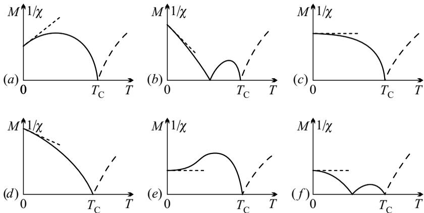
**Fig. 14.16.** Various possibilities for the temperature dependence of magnetization in ferrimagnets. Dashed lines indicate the slope at  $T = 0$ . Above  $T_C$  long-dashed lines show the inverse susceptibility
