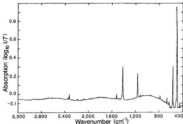
**Fig. 13.1.** Infrared absorption spectrum of an approximately  $2\ \mu\text{m}$  thick layer of solid  $\text{C}_{60}$  on a silicon substrate, referenced to a clean silicon substrate [W. Krätschmer et al., *Nature* **347**, 354 (1990)]
