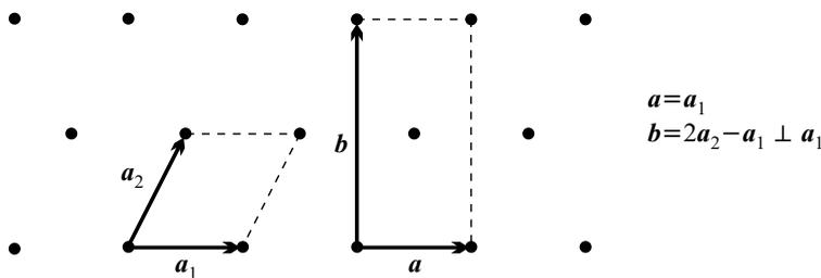
**Fig. 5.9.** The rhomboid-shaped primitive cell and the rectangular Bravais cell of a special oblique lattice
