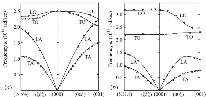
**Fig. 11.13.** (a) Dispersion relations for the lattice vibrations of diamond in two characteristic directions of the Brillouin zone [J. L. Warren et al., *Phys. Rev.* **158**, 805 (1967)]. (b) The same for NaI [based on A. D. B. Woods et al., *Phys. Rev.* **131**, 1025 (1963)]
