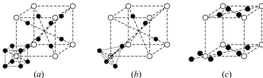
**Fig. 5.30.** Symmetry is either preserved or broken when a simple cubic Bravais cell is decorated with bases of various symmetries. (a) Symmetry of the point group  $O_h$  is preserved. (b) Symmetry is broken to  $T_d$ . (c) Symmetry is broken to  $D_{4h}$ .
