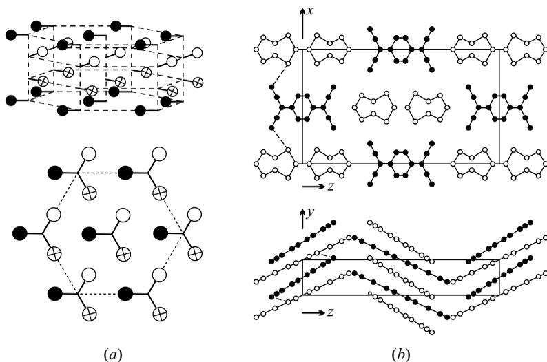
**Fig. 7.24.** (a) The hexagonal A8 structure of  $\gamma$ -Se and its projection on the (001) plane. Atoms marked by  $\bullet$ ,  $\ast$  and  $\circ$  signs are on planes  $c/3$  apart. (b) The projection of the atoms of HMTTF-TCNQ to the (010) and (100) planes
