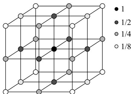
**Fig. 4.3.** The first neutralizing shell around the central atom, and the weights of the ions within. This shell provides the first approximation in Evjen's method for the calculation of the Madelung energy in a sodium chloride crystal
