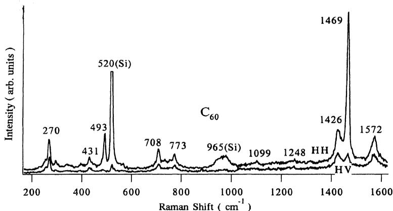
**Fig. 13.6.** Raman spectrum of a thin C<sub>60</sub> layer. Two peaks due to the silicon substrate are observed in addition to the ten Raman active modes [P. Zhou et al., *Phys. Rev. B* **46**, 2595 (1992)]
