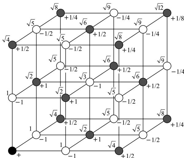
**Fig. 4.4.** Charges in one octant of the shell around the selected ion (bottom left) that have to be taken into account in the second approximation of Evgjen’s method. The numbers above and to the left give the distance of these ions from the central one of the shell, while those below and to the right give their weights within this shell
