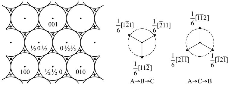
**Fig. 9.16.** The (111) plane through atoms at points 100, 010, 001 in a face-centered cubic lattice. Symbols  $\times$  and  $+$  indicate the centers of atoms in the next ( $B$ -type) and previous ( $C$ -type) layers. The right-hand side shows the vectors that take different layers into each other
