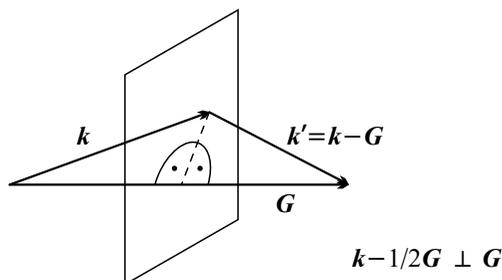
**Fig. 8.3.** Illustration of the Laue condition (8.1.7). The wave vector  $\mathbf{k}$  of the incident beam has to point into the perpendicular bisecting plane of some vector  $\mathbf{G}$  of the reciprocal lattice
