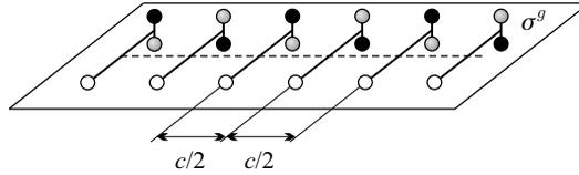
**Fig. 5.28.** Periodic structure with a glide plane
