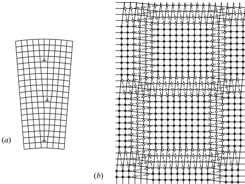
**Fig. 9.23.** Grain boundaries in mosaic structures: (a) tilt grain boundary; (b) twist grain boundary
