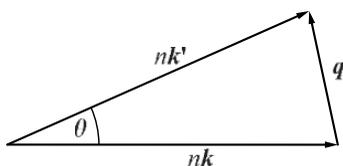
**Fig. 13.8.** The wave vector of the incident and scattered photons in Brillouin scattering
