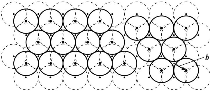
**Fig. 9.20.** Atomic arrangement in the  $(111)$  plane of an fcc lattice above an  $A$ -type layer, when the neighboring  $C$ -type layer is cut and the right part is displaced through  $\mathbf{b} = \frac{1}{6}[\bar{2}11]$
