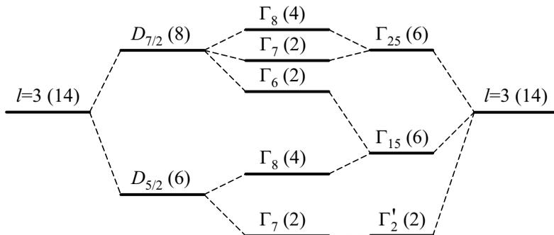
**Fig. 6.2.** Splitting of the 14-fold degenerate energy level of a single electron on the  $f$  shell in a cubic crystal field. On the left-hand side, spin-orbit interaction is taken into account first, and crystal-field splitting second; this order is reversed on the right-hand side. Numbers in parentheses show the degree of degeneracy
