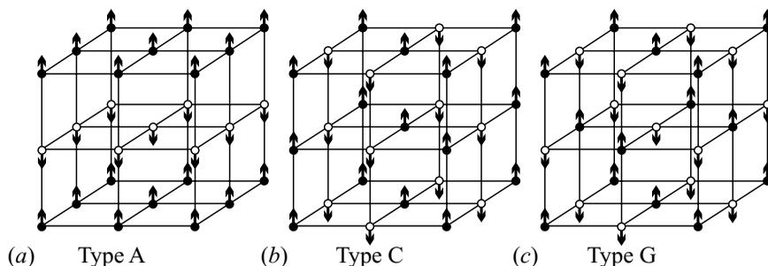
**Fig. 14.2.** Antiferromagnetic structures in simple cubic lattices
