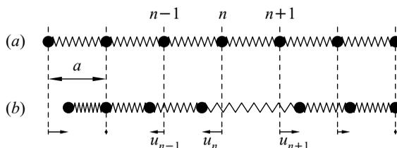
**Fig. 11.1.** Atomic positions in a one-dimensional monatomic chain (a) in equilibrium; (b) in vibration at an arbitrary time  $t$ . Springs represent the elastic forces between the atoms;  $u_n$  is the instantaneous displacement of the  $n$ th atom from its equilibrium position
