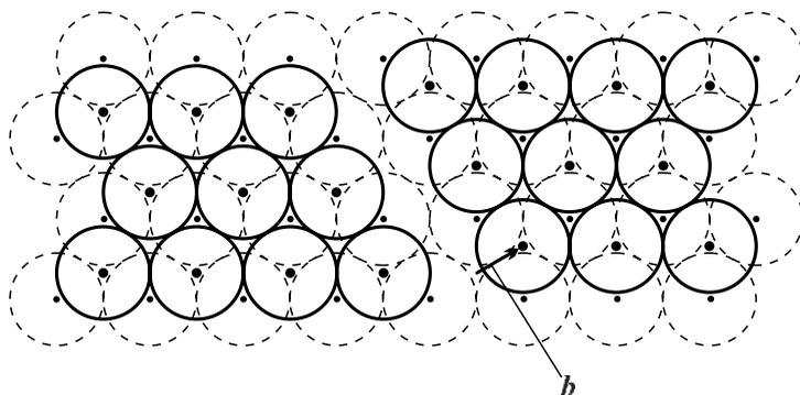
**Fig. 9.18.** Atomic arrangement in the (111) plane of an fcc lattice above an *A*-type layer, when the neighboring *B*-type layer is cut and the part to the right of the cutting edge  $[01\bar{1}]$  is displaced perpendicularly to it, through  $\mathbf{b} = \frac{1}{6}[\bar{2}11]$
