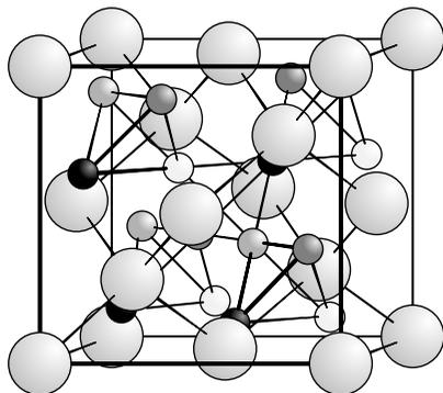
**Fig. 7.17.**  $\text{Cu}_2\text{Mg}$ , the prototype of C15 (cF24) structures
