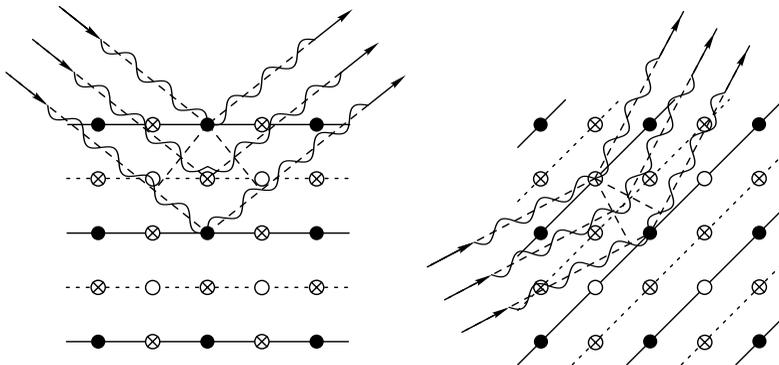
**Fig. 8.7.** Projection of the face-centered cubic crystal onto the plane perpendicular to the  $[001]$  direction, with the  $(100)$  and  $(110)$  planes. Full circles, empty circles and  $\otimes$  symbols indicate atoms at vertices, base centers, and side centers. Solid lines show those members of the family of planes that contain atoms at the vertices of the Bravais cell. Atomic planes drawn with dashed lines are the result of centering
