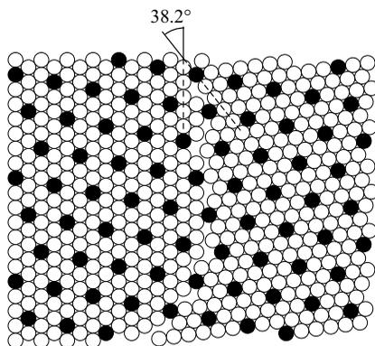
**Fig. 9.25.** Coincident-site lattice in the close-packed plane of a face-centered cubic crystal formed between two grains with a relative orientation of  $38.2^\circ$ . The atoms marked by full circles exhibit regular crystalline order
