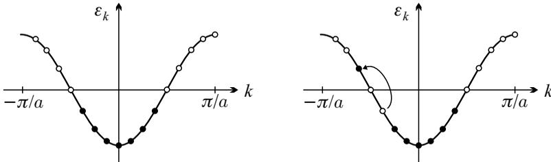
**Fig. 15.14.** Wave numbers of free spinless fermions in the lowest-energy state of the  $S_{\text{tot}}^z = 1$  sector and in a possible excited configuration for  $N = 16$  and  $N_{\downarrow} = 7$ . Occupied sites are indicated by full circles
