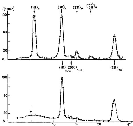
**Fig. 14.5.** Neutron-diffraction pattern of MnO: (a) in the low-temperature antiferromagnetically ordered phase at 80 K; (b) in the magnetically disordered phase at room temperature. The extra peaks that appear in the magnetic phase are satellites [C. G. Shull, W. A. Strauser, and E. O. Wollan, *Phys. Rev.* **83**, 333 (1951)]
