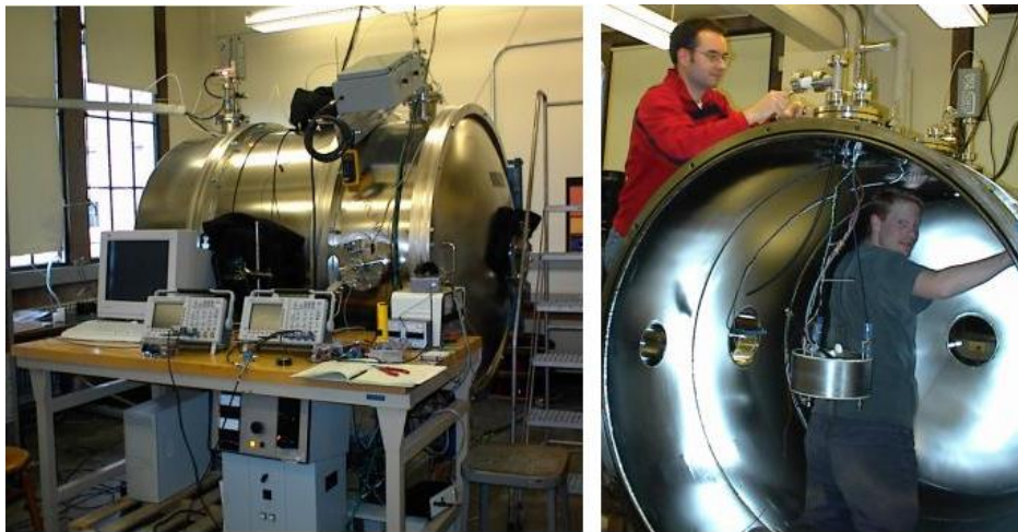
Figure 7: 4000 L prototype test chamber at the University of Washington (figure courtesy of official M2P2 website).
