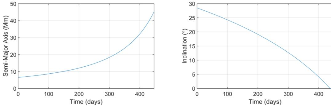
Figure 4. Semi-Major Axis and Inclination for Low-Thrust Transfer to GEO.
