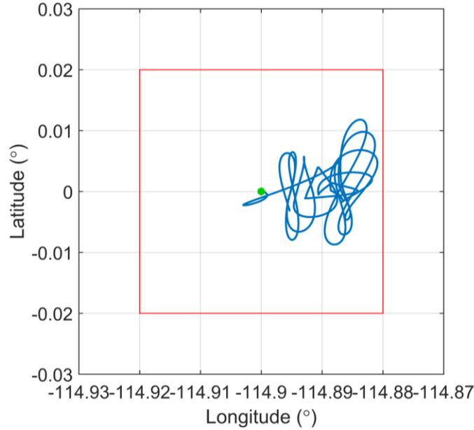
Figure 7: Longitude and Latitude of Satellite with Chemical Thruster
