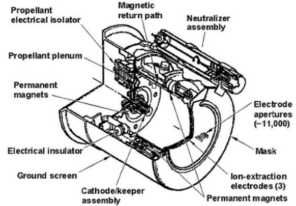
Figure 2. Schematic of XIPS thruster.<sup>[5]</sup>
