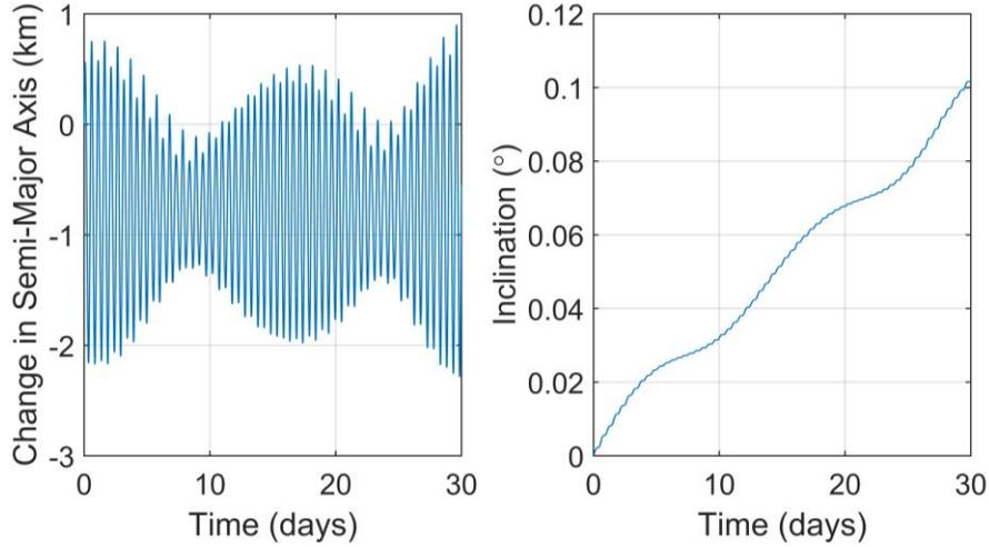
Figure 6: Changes in Orbital Elements Due to Perturbing Accelerations.
