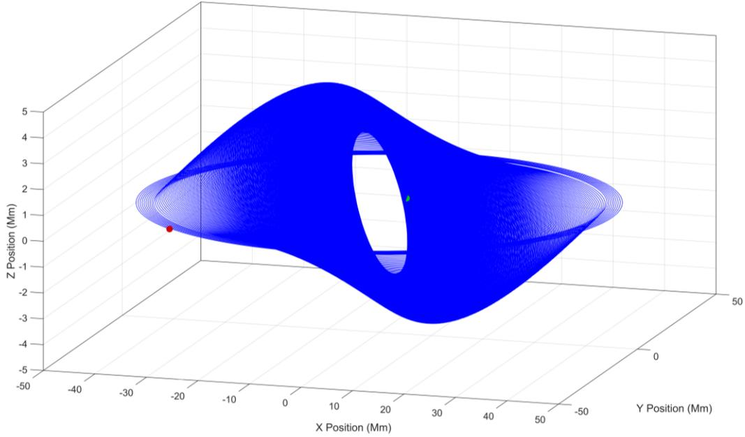
Figure 3. Trajectory for Low-Thrust Transfer to GEO.
